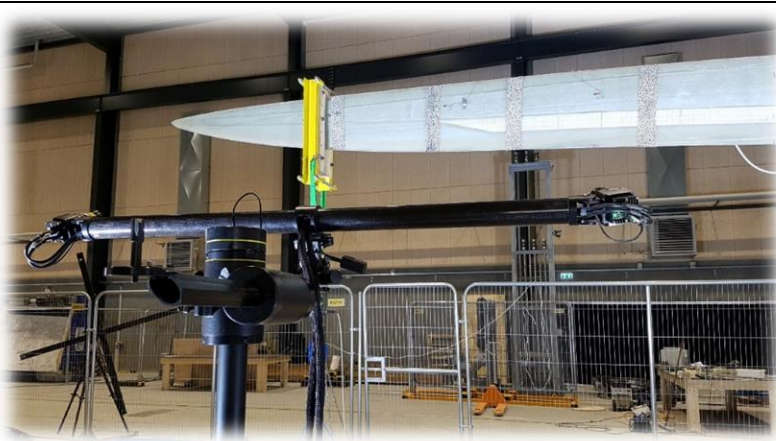
Figure 5.3.5. Digital Image Correlation (DIC) setup used to measure the displacement field during the BPE test campaign
