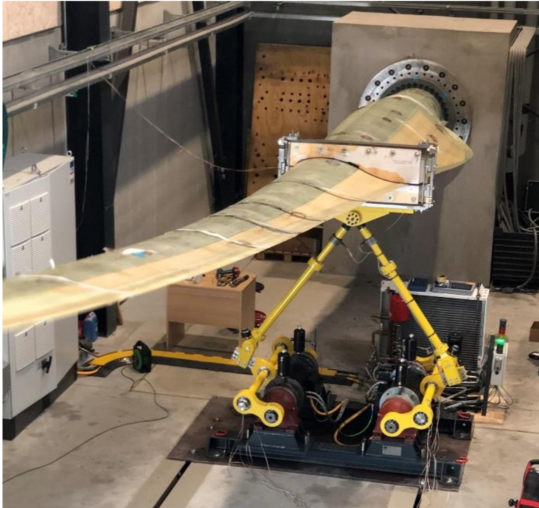
Figure 5.5.8 – Dual axis exciter version 2 with backlash-constrained drivetrain installed at DTU Large-Scale facility during test.
