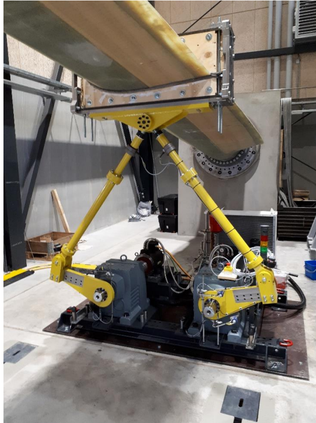
Figure 5.5.4 – Version 1 of the Small Dual Axis Exciter mounted with 14m blade at the DTU test facility
