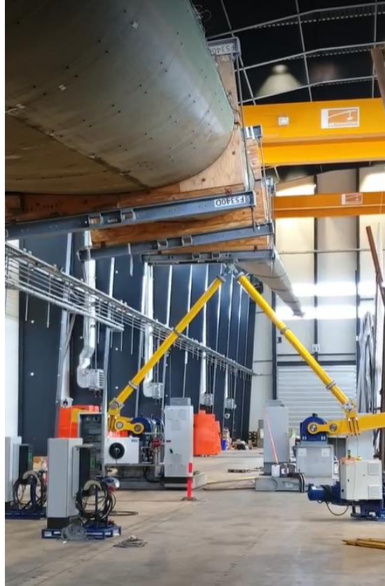
Figure 5.7.3. Example of test set-up for B75 blade demonstration.
