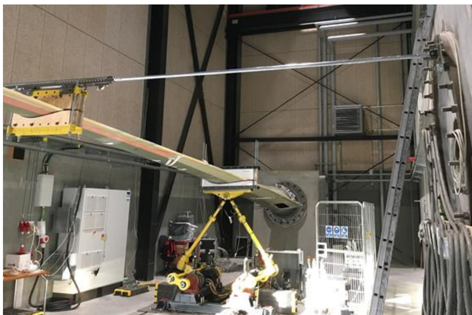
Figure 5.5.10. Test set-up, OW1430 blade, R&D exciter and 1D-mass (rail only, no added mass). Load saddle is located at 5,2m, the 1D-mass saddle at 10m.
