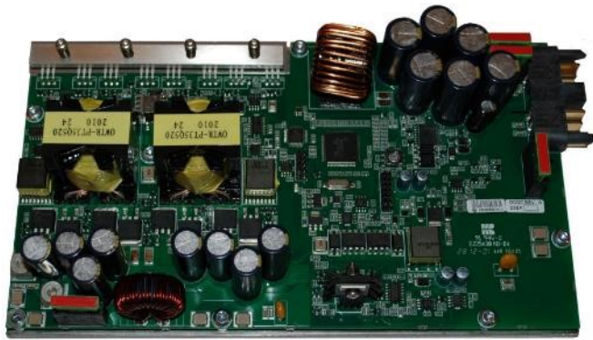
Figure 18 DCDC converter currently used in BPSE Stationary fuel cell applications
