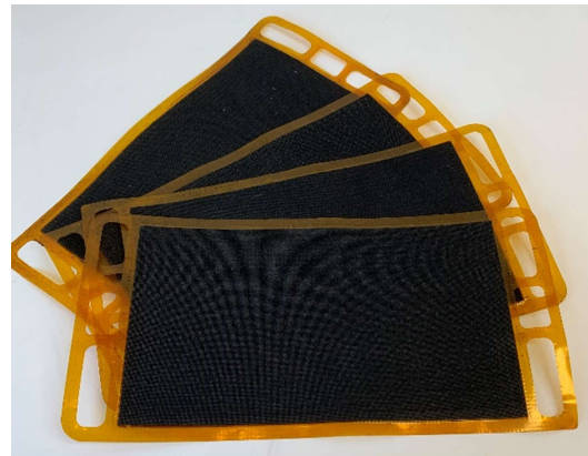
Figure 26: HTPEM MEAs in the 165cm 2 format used in SereneU systems assembled in Aalborg
