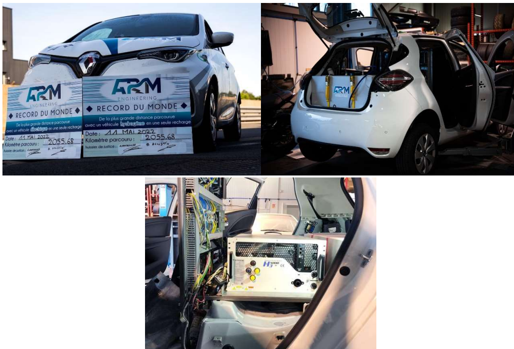
Figure 62: Breaking records! Electric Renault Zoe running 2000km before requiring charging. Using Advent 5kW HTPEM fuel cell system.
