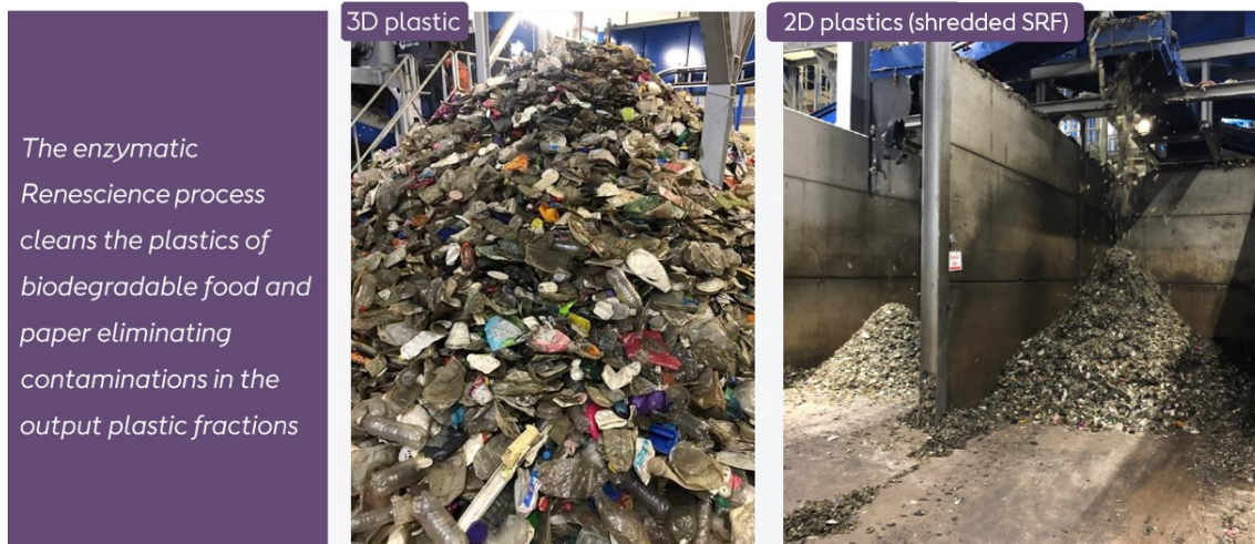
Figure 6 - 3D and 2D plastic fraction produced at the full-scale demonstration plant, Renescience Northwich.
