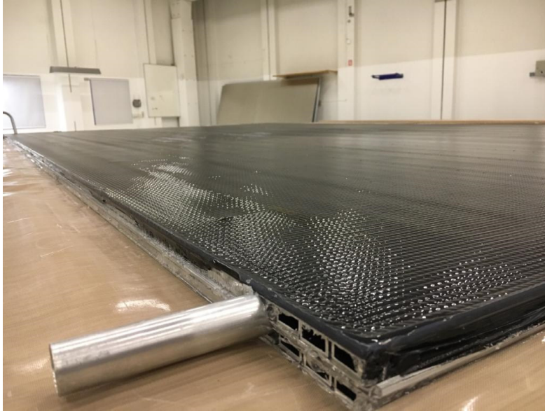
Figure 3.2.2 (II) The header pipe is well hidden, but at the cost of some very heavy hand made aluminum sandwich construction
