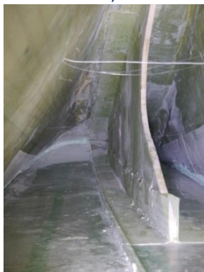
Figure 12: A) and B) Prototype #1 and #2 are both designed to be retrofitted in a SSP34m blade. For each prototype, experience is gathered and used in the design for the next prototype. C) The Floor™ prototype are retrofitted in the LM58.7m blade which are almost twice as long as the SSP34m blade.
