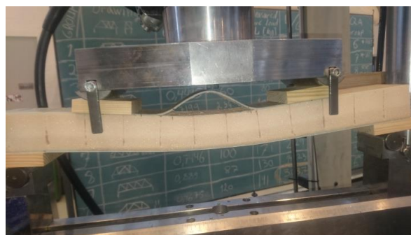
Figure 37: Detail of the face buckling under compressive state loading. This is phenomenon additionally lowers the bending stiffness of the setup
