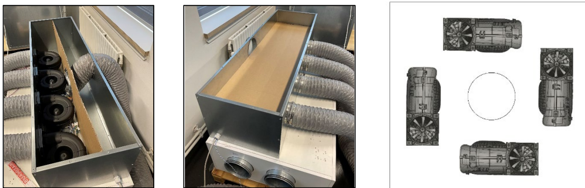
Figure 17. Current prototype of the air distribution box in the Ebm-papst laboratory (left & middle), the expected final “square” design (right).
