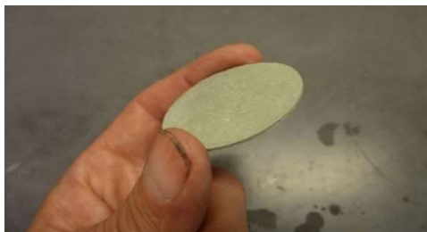
Figure 9 Ø42 mm electrolyte disk consisting of \text{CsH}_2\text{PO}_4 with \alpha\text{-SiC} filler
