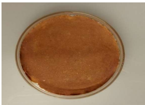
Figure 10 Cast electrolyte, containing \text{CsH}_2\text{PO}_4 and \text{SiC} filler. \text{Ø} >100 mm
