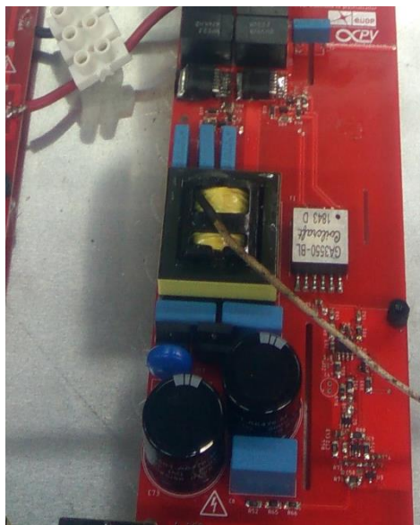
Figure 1. Picture of the LLC transformer used as slave module in the grid-tie inverter
