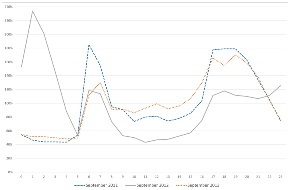
Figure 2: Load profiles of the households with an EV for 2011-2013 for weekdays in June and September. Note: Hours shown on X-axis are in Danish Summer Time. 100% represents the average hourly load of the sample.
