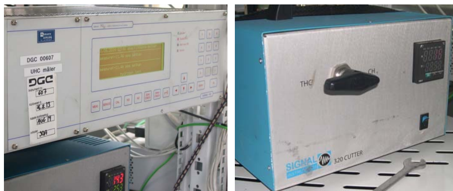
Figure 13 FID analyser and non-methane cutter used by Danish Gas Technology Centre
