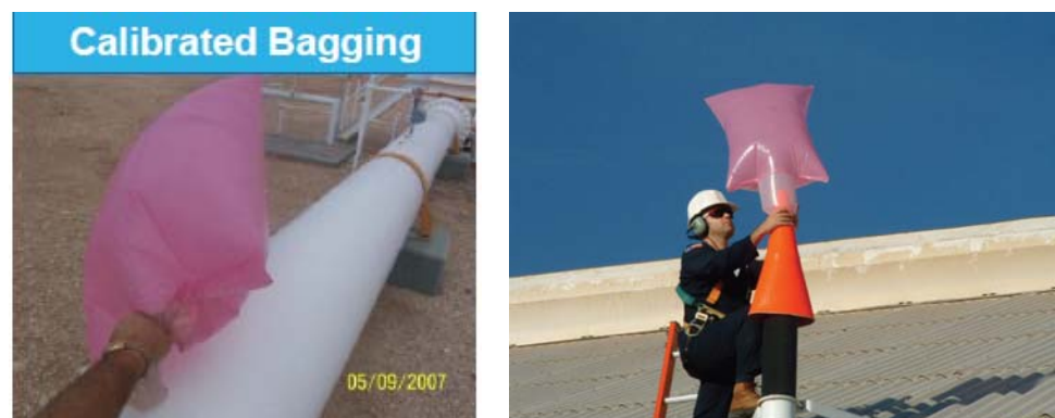
Figure 5 Quantifying emissions using calibrated bagging
