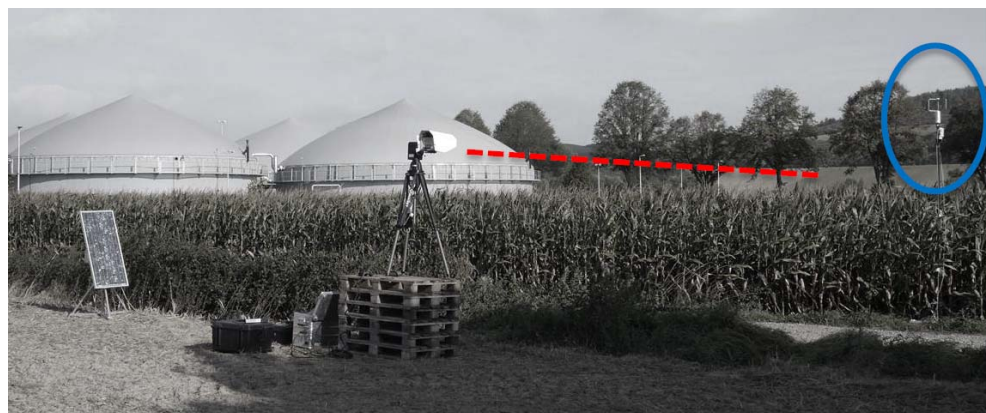
Figure 2 Quantification with TDLAS and inverse dispersion modelling (Source: DBFZ)
