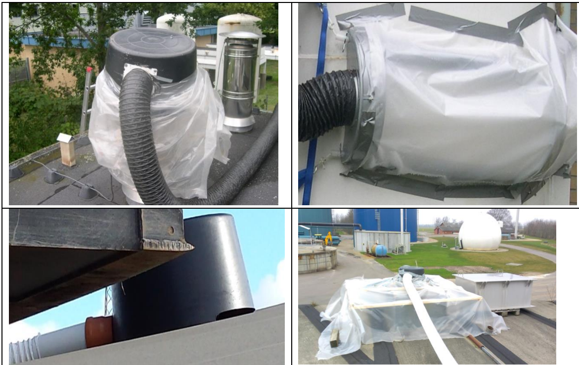
Figure 4. Examples of sampling devices suited for measuring methane leakages. Top left: Sampling device suited for leakages from pressure relief safety valves. Top right: sampling device for measurement of a leakage on a curved surface. Bottom left: sampling device for sampling a leakage in biogas digester cover. Bottom right: Sampling device designed for measurement of methane emission from a mixing pump cover box situated above a digestion tank.
