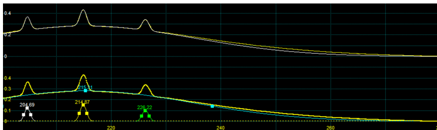
Figure 4.3: Spectral deconvolution in the 200-280 nm spectral range using PeakFit. Manual optimisation has been performed to achieve the best possible fit (least squares method). The individual spectral components can be seen from the bottom half of the screen, whereas the top half shows the cumulative simulated spectrum (white) and the experimental spectrum (yellow).
