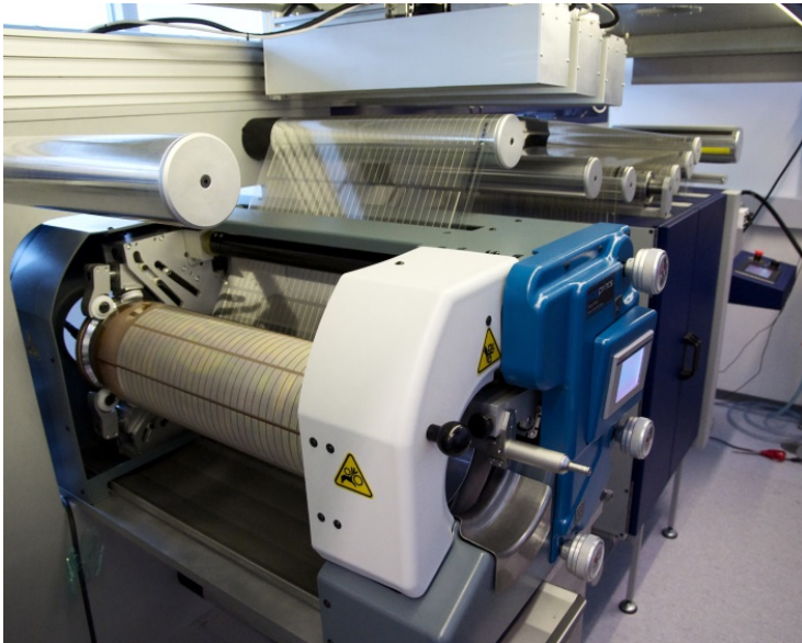
Fig 1. Rotary screen printing of PEDOT:PSS electrodes on the 510 mm wide machine
