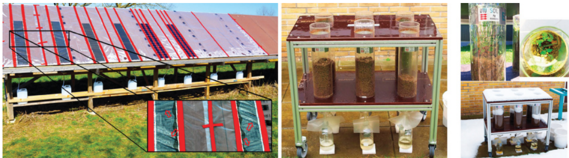
Fig 25. Left: Rain run-off leaching setup with different silver and carbon-based solar foils, either intact or damaged on purpose. Right: mobile soil sequestration/leaching setup with solar foil buried in soil, either intact or shredded.
