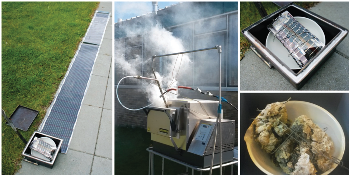
Fig 27. Left: Picture of 1 m 2 of an organic solar cell rolled out on the ground. On the bottom left of the same picture an additional 1 m 2 has been cut into smaller pieces, tied up with heat resistant steel wire and put in a ceramic bowl inside the steel container. Middle: Picture of the oven setup with the steel container placed inside the high temperature oven with a controlled air flow. Right: Pictures of the cut up solar cells before and after incineration.
