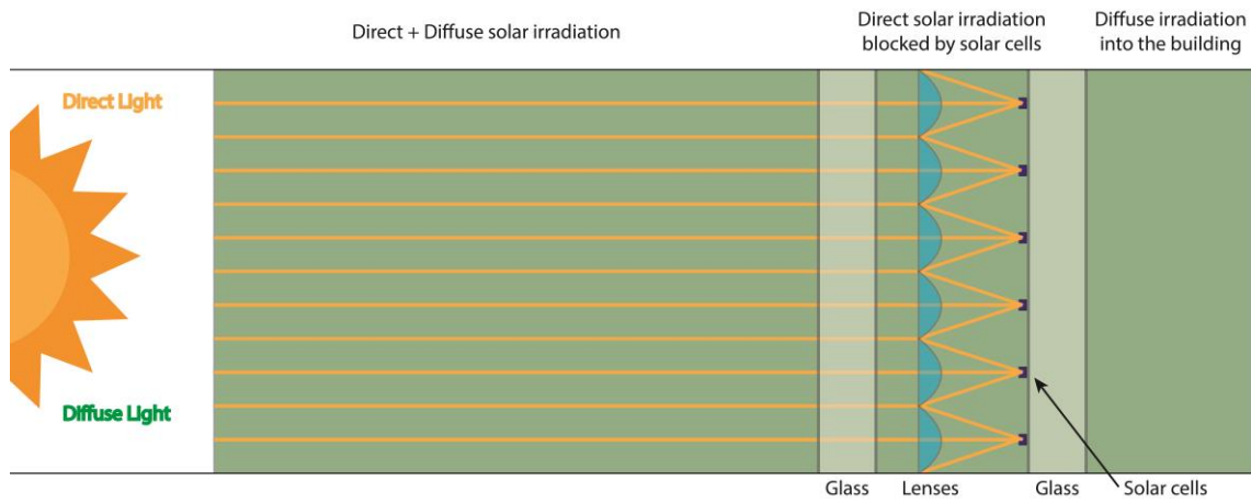
Figure 3 - BICPV principle evaluated in the project. Direct light is concentrated by cylindrical lenses onto solar cells and blocked/harvested while the diffuse light penetrates into the building.
