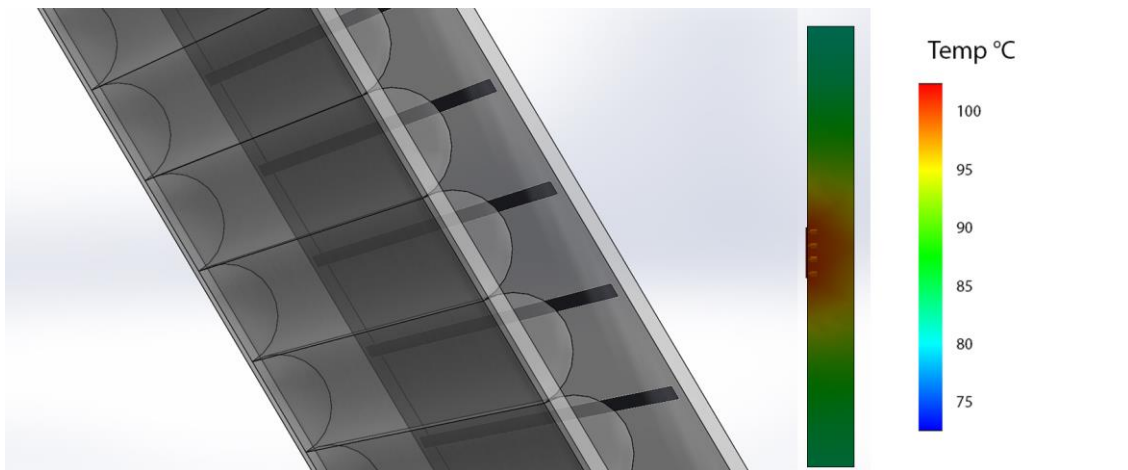
Figure 17 – Coarse thermal simulations using glass as substrate seen in cross section.
