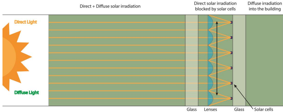
Figure 20 – Side view of the proposed BICPV concept
