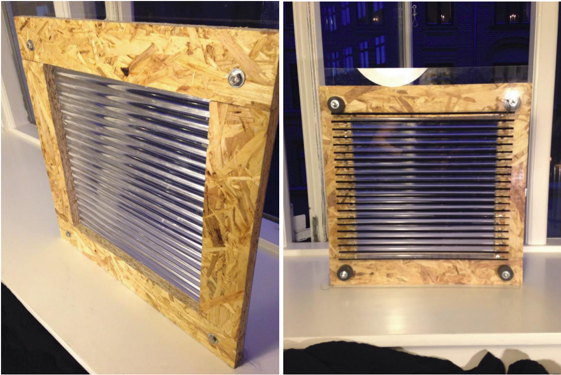
Figure 21 – Demonstrator of the Lens / PV line principle. Left: Front side towards the sun with the lens exposed. Right: View from the back-side of the system. The black lines illustrate the solar cell lines.
