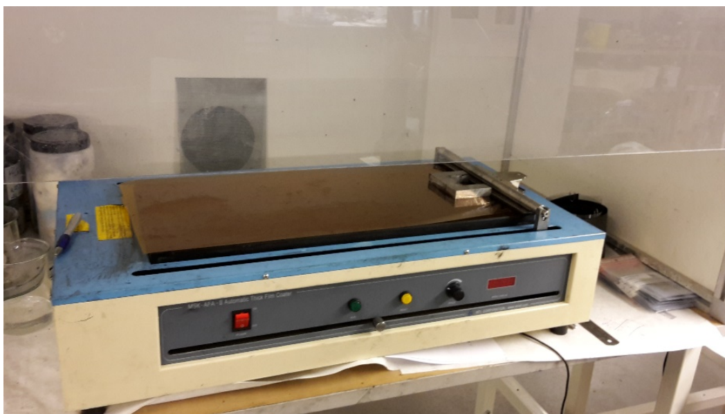
Figure 12. Table top tape casting equipment for development of new electrode production method.
