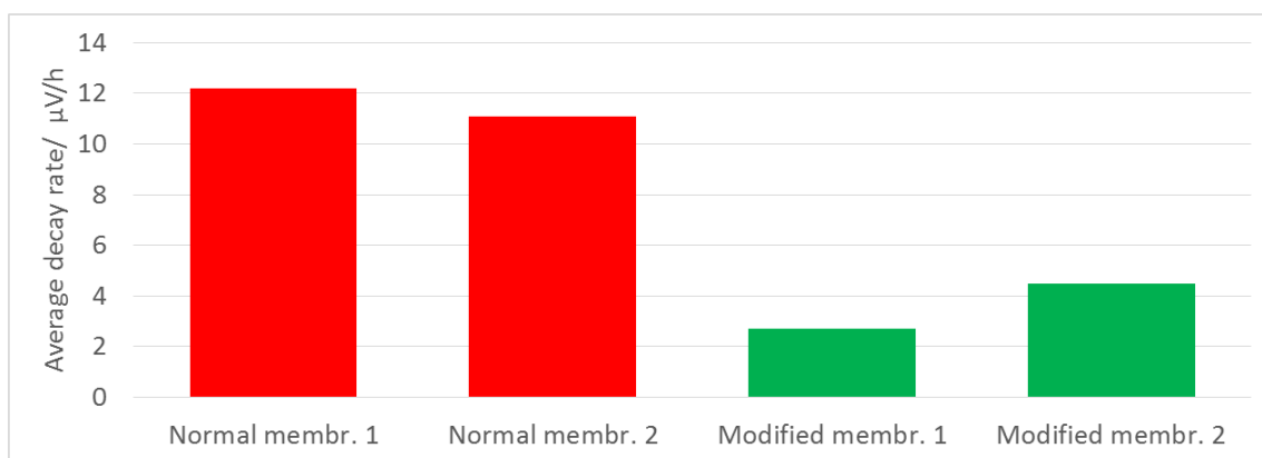
Figure 25. Decay rates over several thousands of hours at 180 °C for test cells with two normal PBI membranes and two modified membranes.
