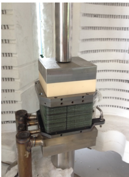
Figure 3 - SOFC stack used for the project
