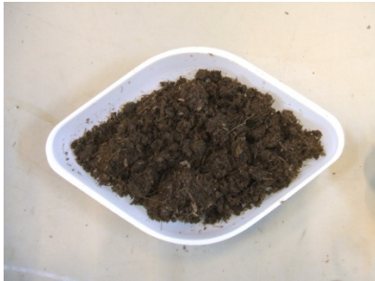
Figure 18 – Morsø Bioenergi AD fiber
