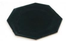
Figure 8 The PVD aluminium nickel plate after heat treatment and selectively etching of aluminium
