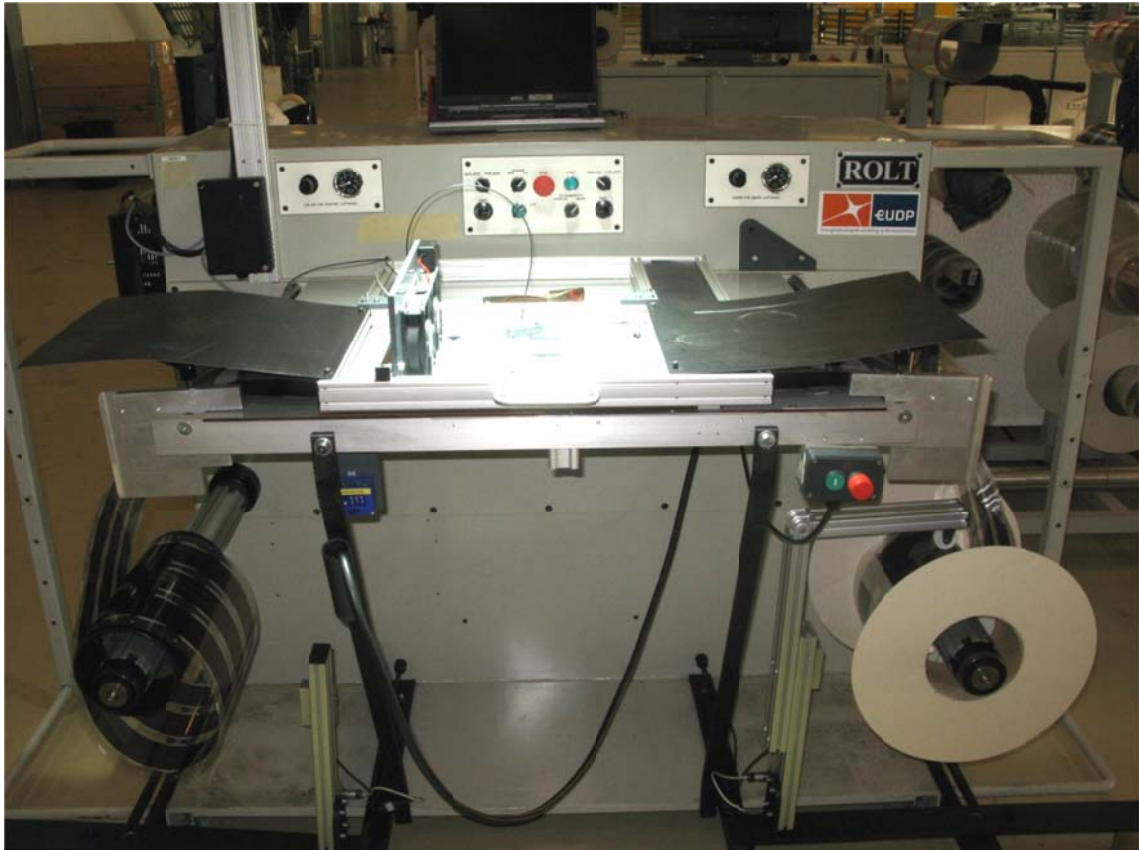
Figure 3-4: Automatic R2R-tester for full characterization of solar cells produced.
