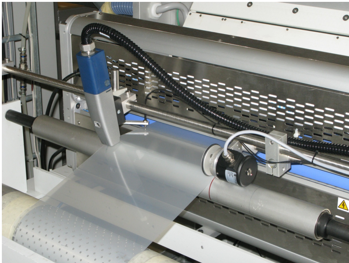
Figure 3-1: Ink-jet printer writing barcodes for tracking of process parameters and performance
