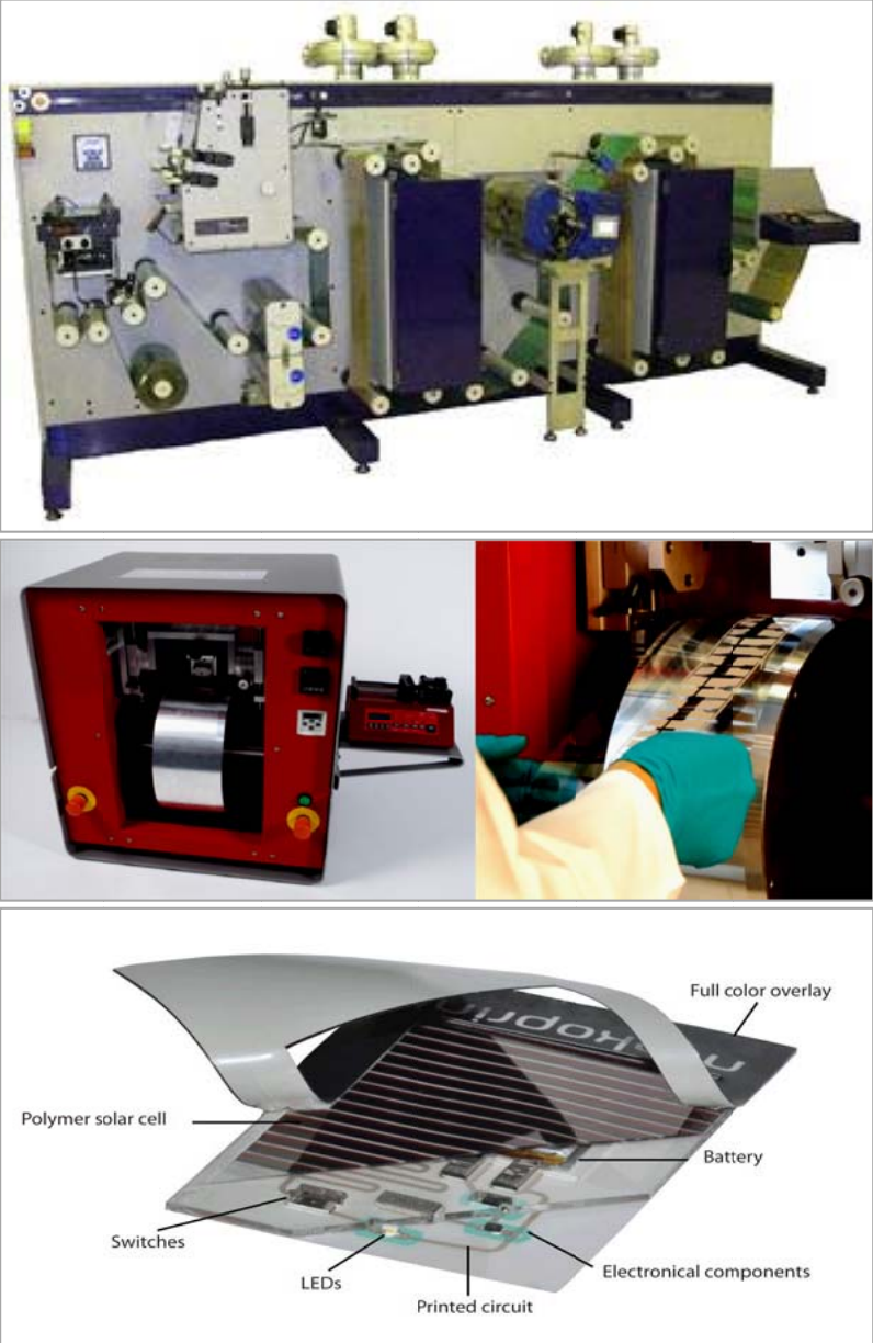
Figure 6-1: Example of commercially available OPV product: a roll-to-roll coating/ printing machine from Grafisk Maskinfabrik (top), a mini roll coater for OPV R&D purposes developed by DTU and sold by FOMTechnologies (middle) and an OPV flash light sold by Mekoprint (bottom).
