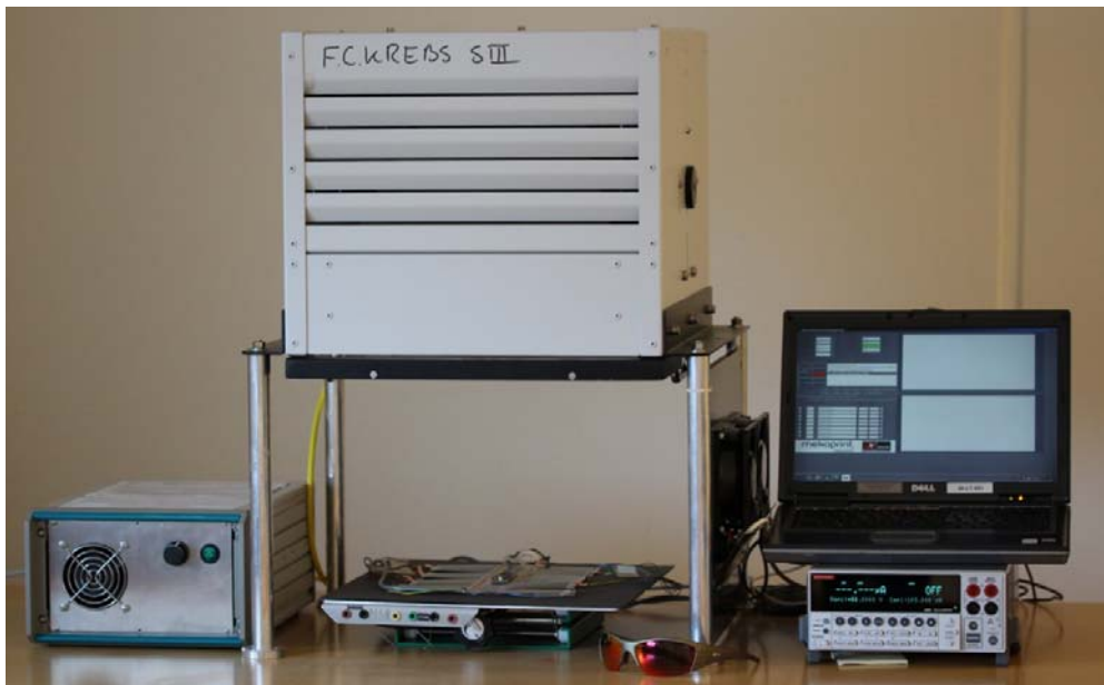
Figure 3-3: IV-test stand with multichannel 4-point IV-trace and life time measurement.
