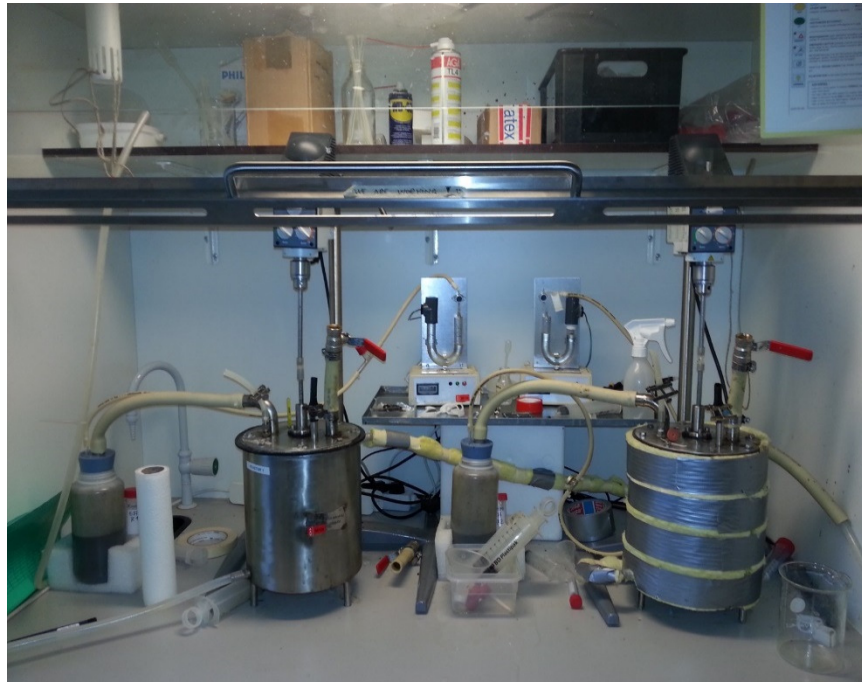
Figure 4: Verification of the AD-Booster effect with bench-scale reactors at AAU
