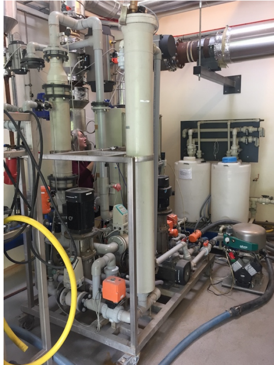
Figure 23 Picture of the ceramic UF system from LiqTech
