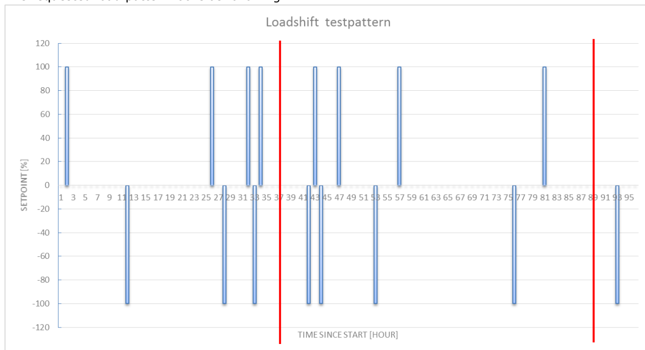
Figure 51: Graph of loadshift testpattern with delivery positive, and consumption negative. Pattern of 4 days (96 hours). The red lines illustrates the period identical to the performed test below.
