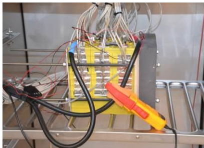
Figure 90: Cell Pack test in climate chamber
