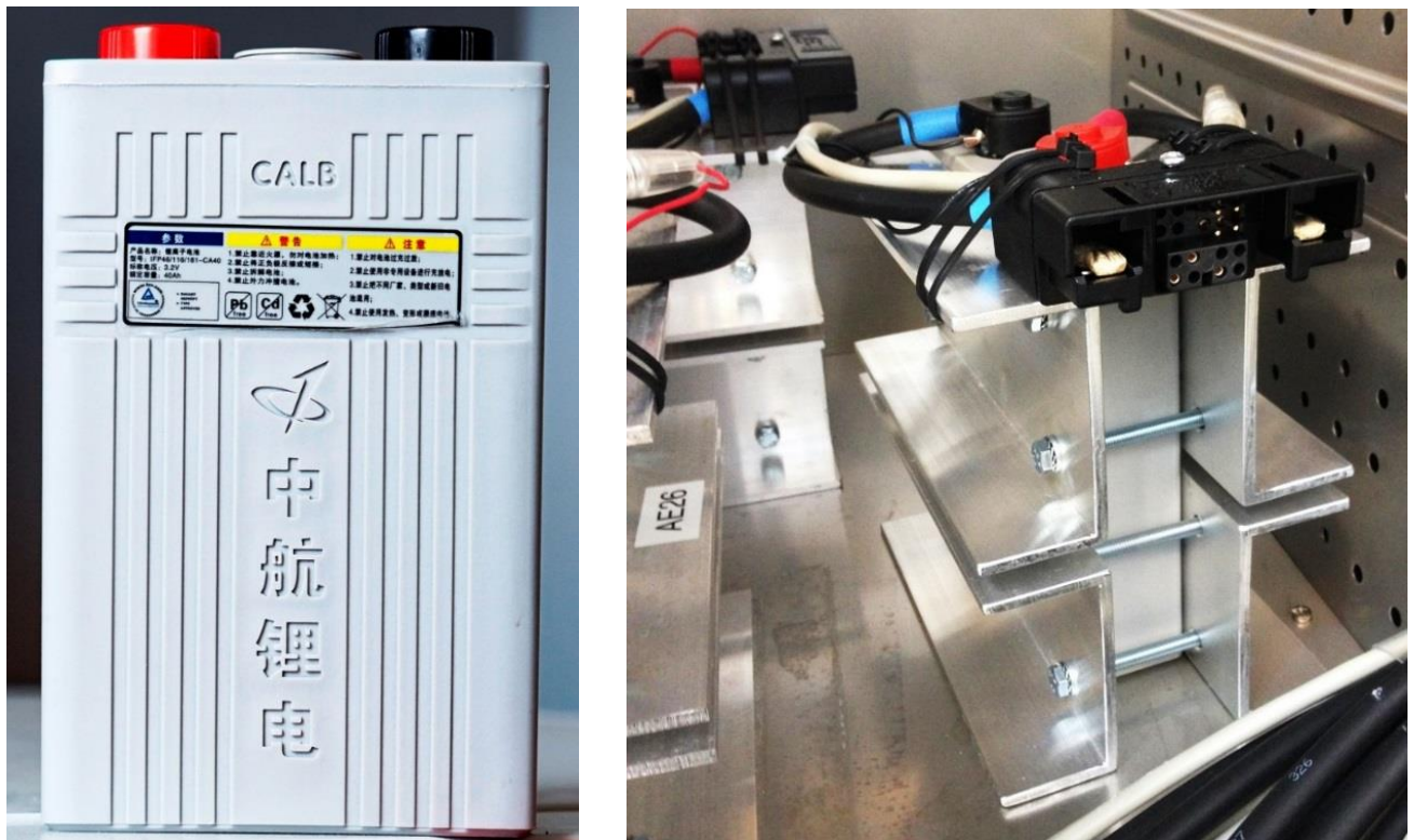
Figure 94: CALB cell and test fixture
