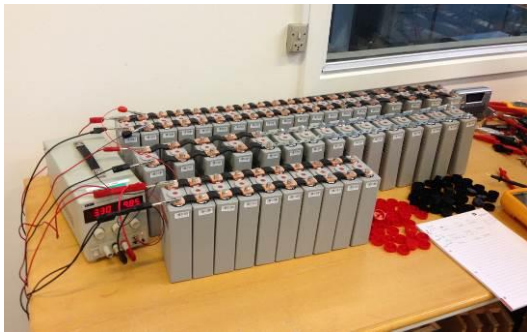
Figure 91: Initial charge of 40Ah Lithium-Ion cells for single cell degradation tests
