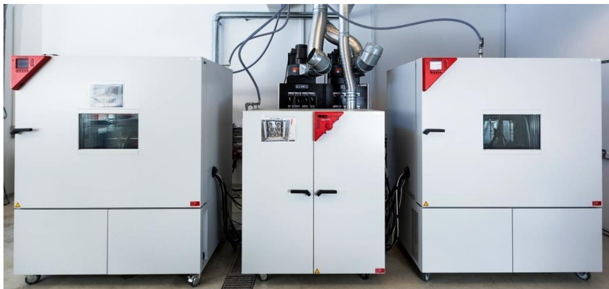
Figure 95: Binder chambers and Maccor 4000 Battery tester in the background
