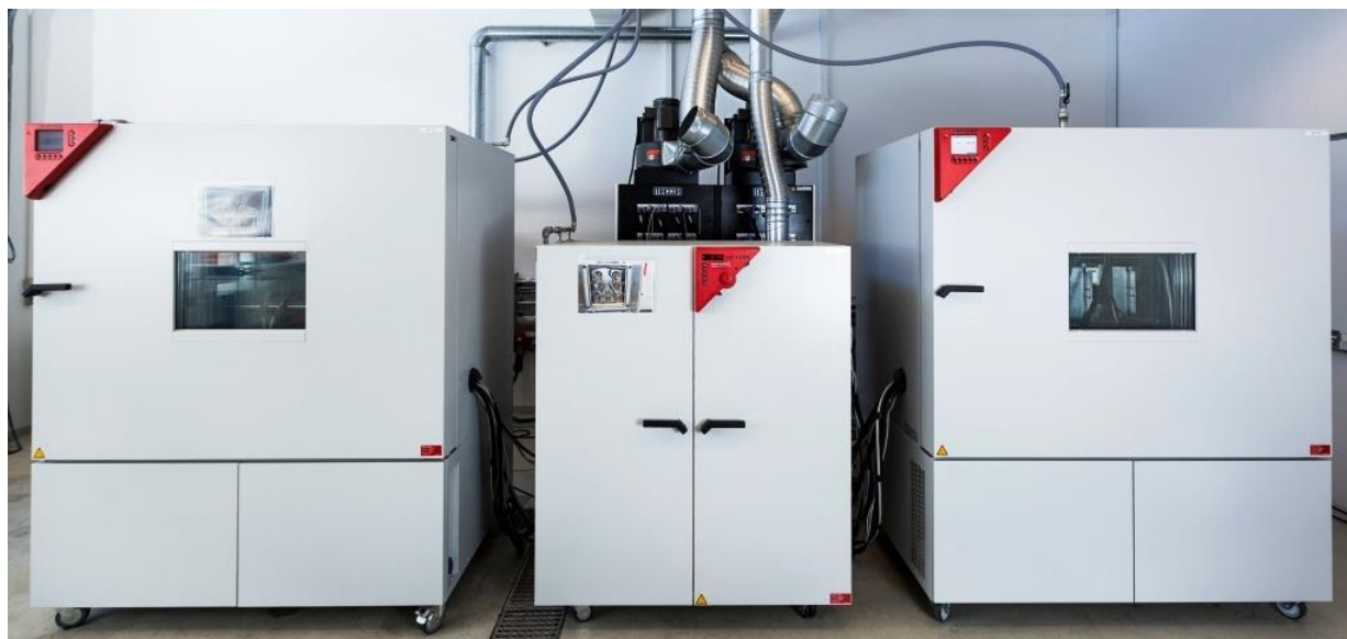
Figure 29: Binder chambers and Maccor 4000 Battery test system in the background
