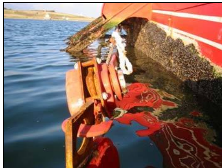
Fig. 8.5 Blue mussels seen growing around the structure
