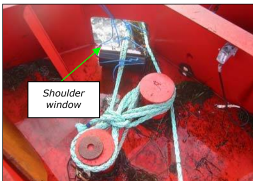
Fig. 4.3 Rubbing at shoulder window
