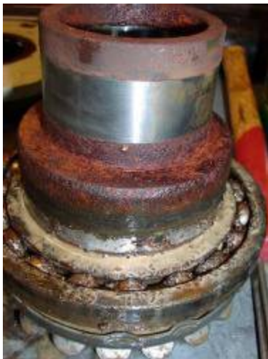
fig. 3.2.: Corroded components of a turbine bearing.
