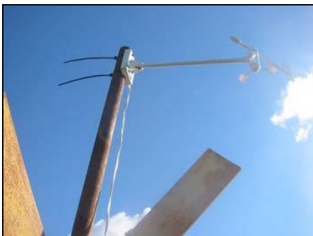
Fig. 2.3 Wind vane mounted on mooring pile
