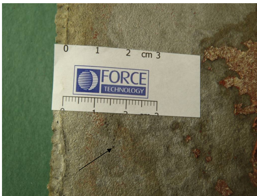
Figure 11 Pitting 0.2 mm deep in sample 2 after acid cleaning.
