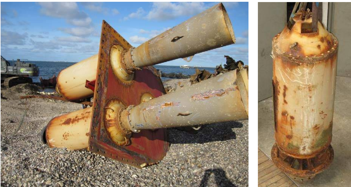
fig. 3: turbines on the beach during dismantling of the WD structure and one of them on arrival in Munich
