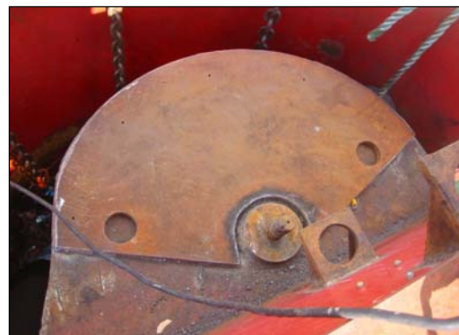
Fig. 5.16 Modified fishtail plate
