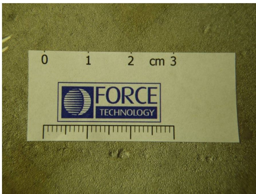
Figure 9 Pitting 0.6 mm deep in sample 1 after acid cleaning.
