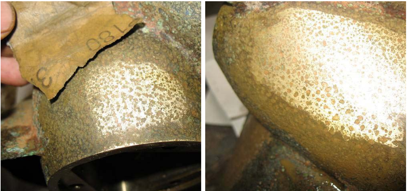
fig. 35: corrosion on turbine runner
