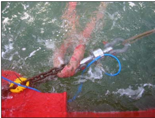
Fig. 2.7 Force transducer as originally installed
