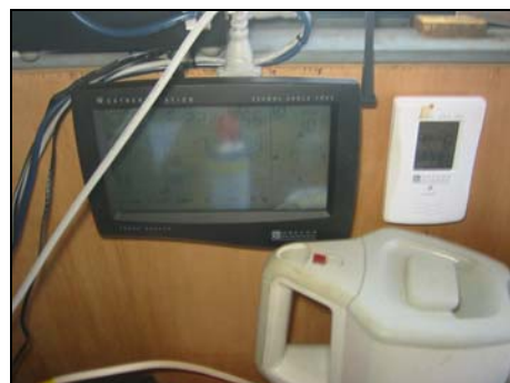
Fig. 2.6 Indoor temperature/humidity/air pressure sensor/panel
