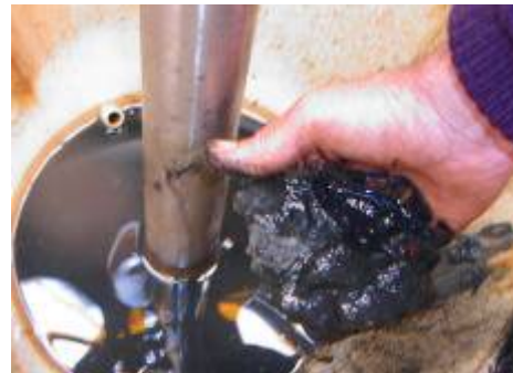
fig. 3.4.: Sand-filled water-lubricated bearing
