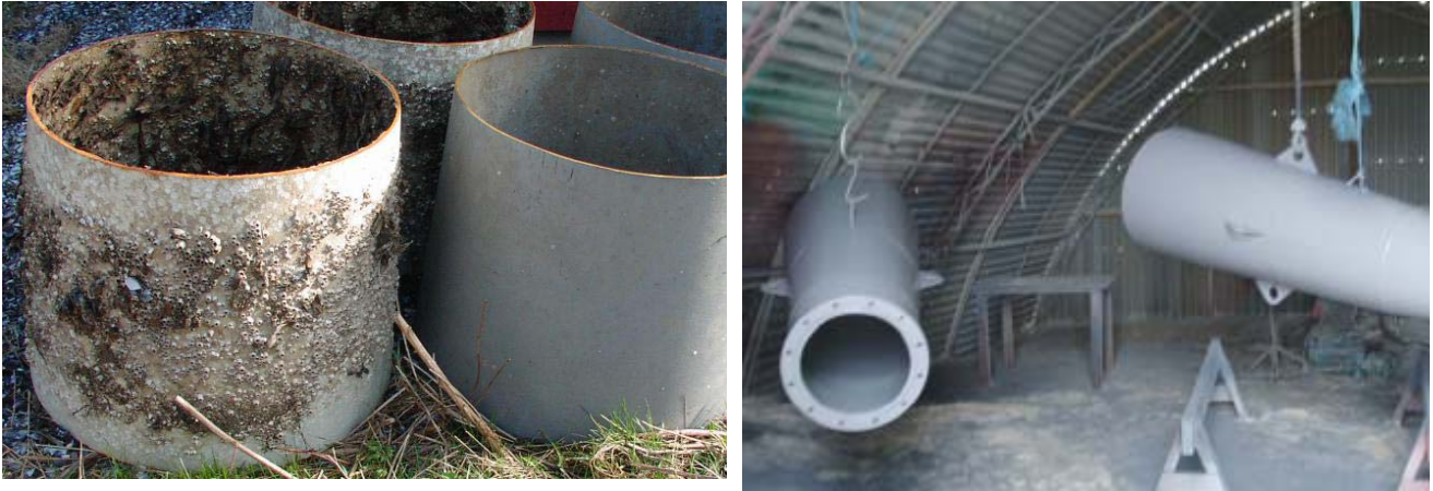
fig. 40: draft tube sections with epoxy and silicone paint
