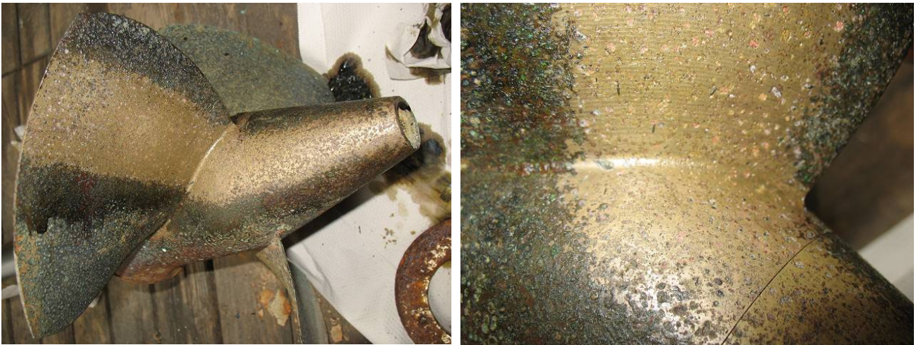
fig. 34: corrosion on turbine runner
