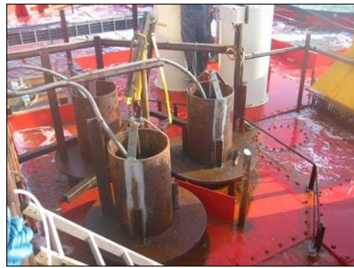
Fig. 3.9 Dummy turbines following maintenance
