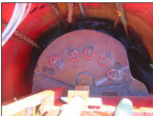
Fig. 5.17 Fishtail plate with chain rings welded
