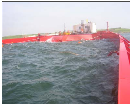
Fig. 5.6 Wave Dragon with reflectors re-installed
