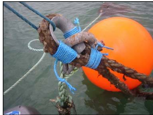
Fig. 4.7 Improved mooring line protection
