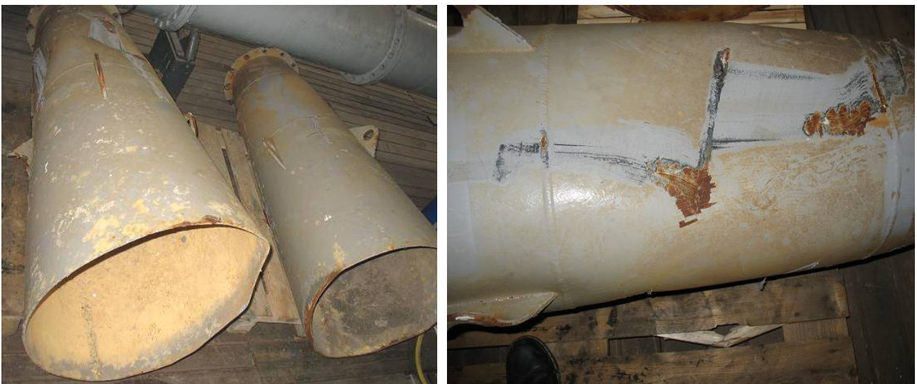
fig. 41: draft tubes with silicone paint system
