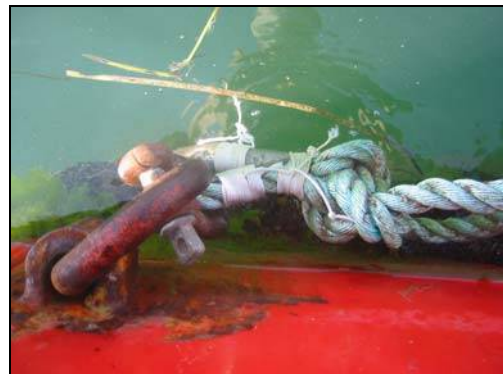
Fig. 4.9 Improved thimble/shackle mooring arrangement
