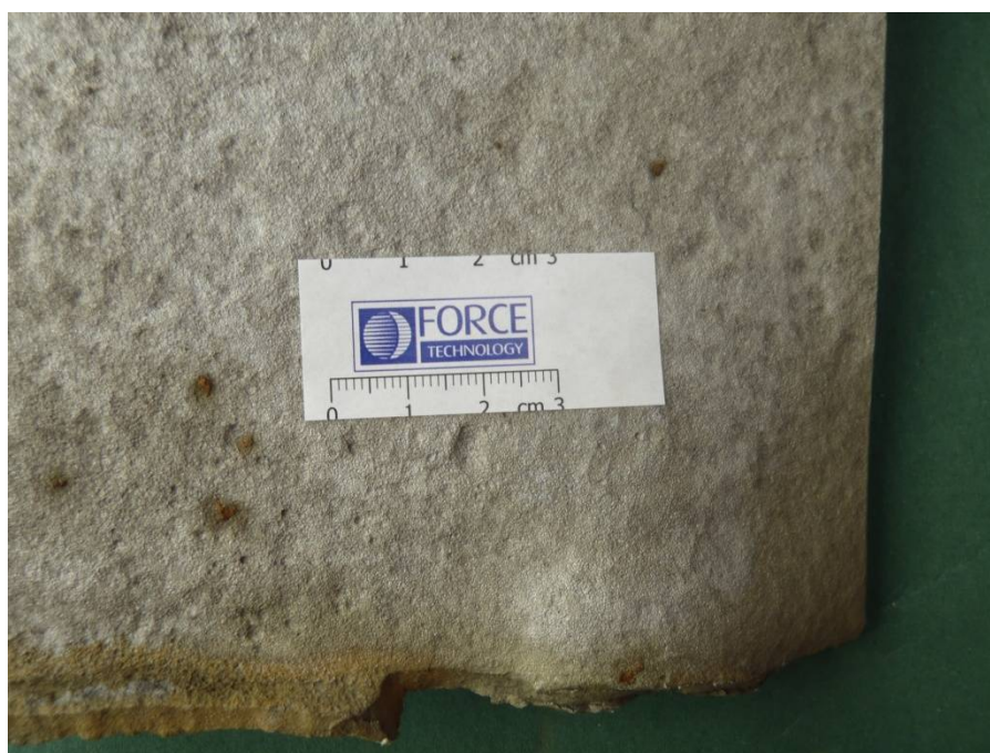
Figure 13 Pitting 1.1 mm deep in sample 3 after acid cleaning.
