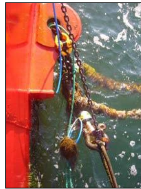
Fig. 2.9 Force transducer wire failure
