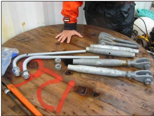
Fig. 4.1 Mooring equipment for deflecting lines from rear of WD
