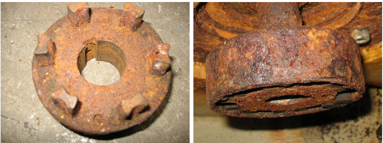
fig. 17: generator shaft coupling
