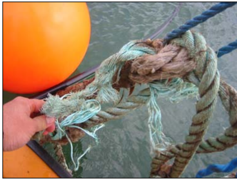
Fig. 4.6 Significant wear on starboard reflector mooring line
