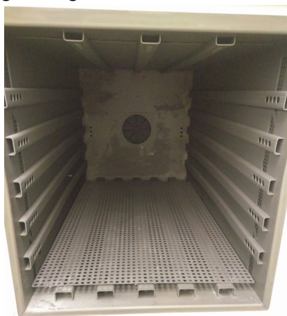
Figure 7: Interior of the large furnace for production of 1:1 sized foam glasses.
