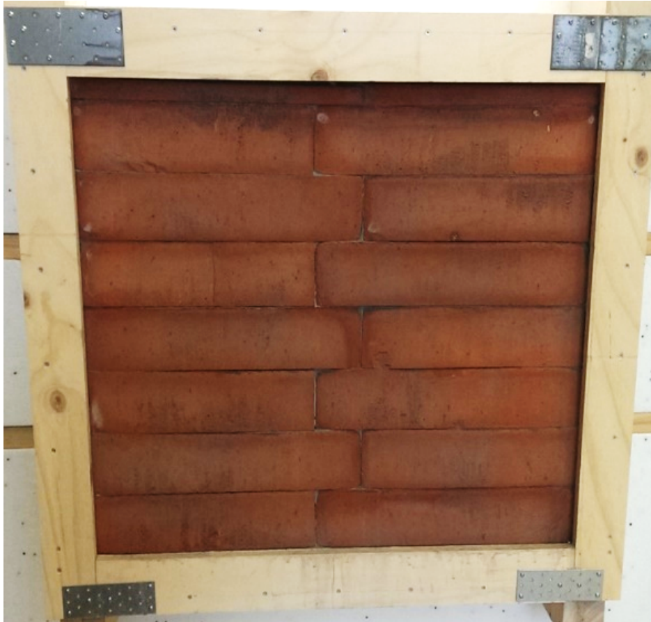
Figure 12: CleanTechBlock wall element mounted on insulation frame for Guarded Hot Box test.
