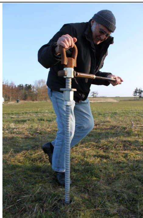
Torque app. : 50 kg x 1 m = 500 Nm
