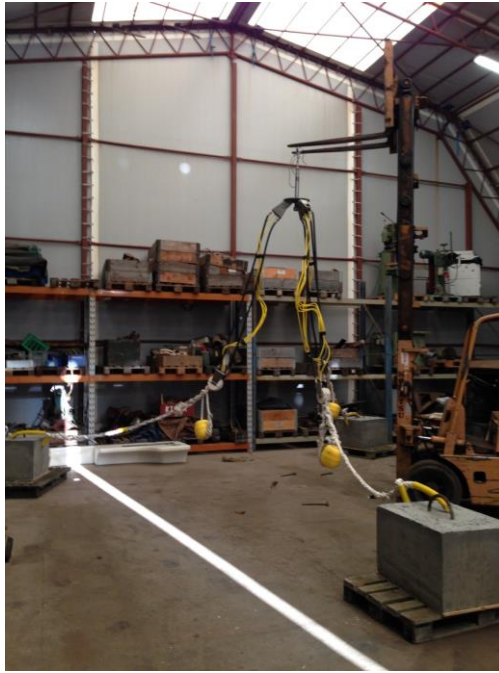
Figure 22 Complete mooring system assembled on land
