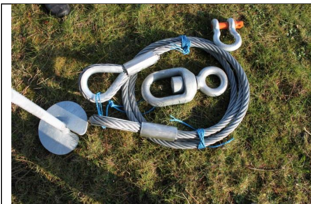
Typical selection of mooring wire and shackles for 10 ton operation
