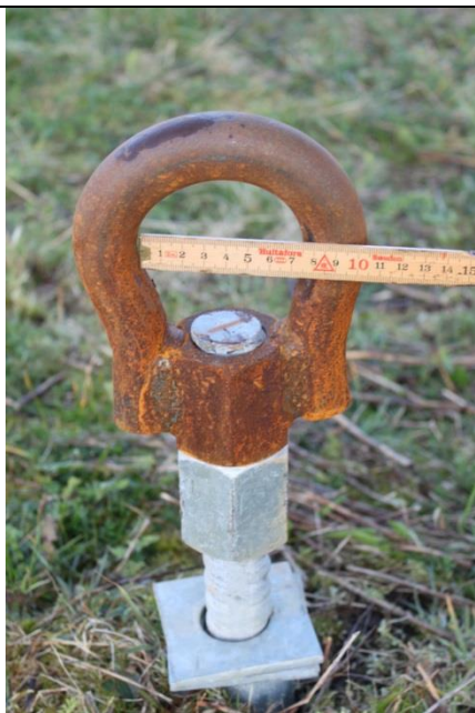
The screw anchor installed to 2m depth
