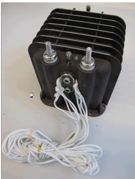
Figure 3. The new APU stack. Weight 10 kg. Dimensions are 184 x 159 x 166 mm. Two threaded power outlets are seen. Voltage probes leave from the side. Depending on the fuel, the duration of operation and efficiency trade-offs, each stack can deliver an electrical power in the range 2-3 kW.
