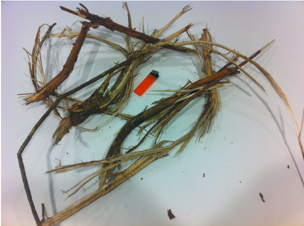
Picture 17: Willow tweaks that had coiled up in the gasifier during test run.
