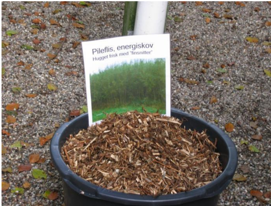
Picture 13: Willow chips supply from HedeDanmark. The willow chips were made from freshly harvested material using in fine chopper equipment.
