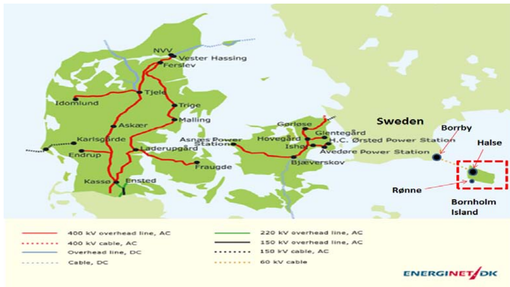
Figure 1-1 Map of Danish transmission system and Bornholm distribution system in red dotted box at the right corner (EnerginetDK Website)
