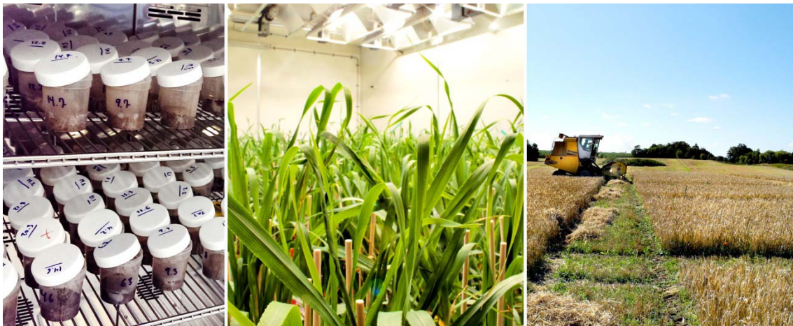
Figure 3: Investigation of Pyroneer ash quality in laboratory scale incubation studies (left), pilot scale pot plant experiments (center) and demonstration scale field trials (right)
