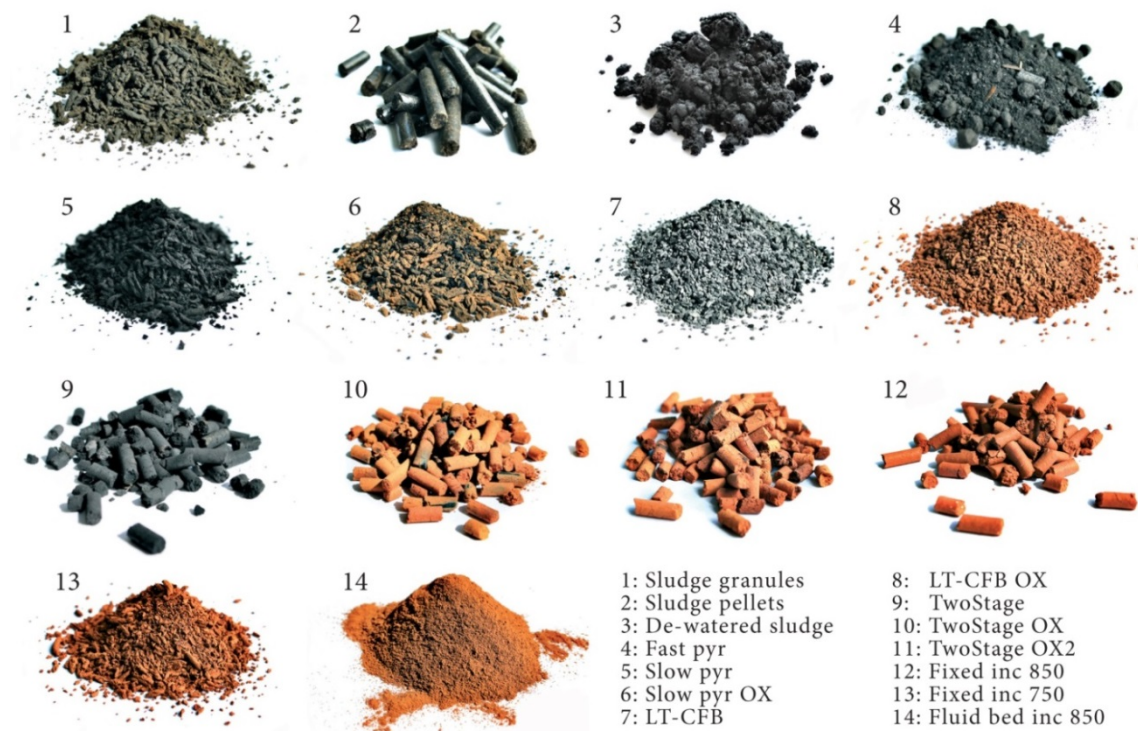
Figure 7: Pictures from the CPSE study of sludge fuel variants (1-3) obtained from the Danish WWTP Bjerghmarken Renseanlæg in Roskilde as well as of ash and char substrates from pyrolysis (4-5), gasification (7,9), and incineration (12-14) of the sewage sludge samples. Post oxidized samples of slow pyrolysis char (6), LT-CFB bottom ashes (7) and TwoStage gasifier ashes (10-11) were also included in the study
