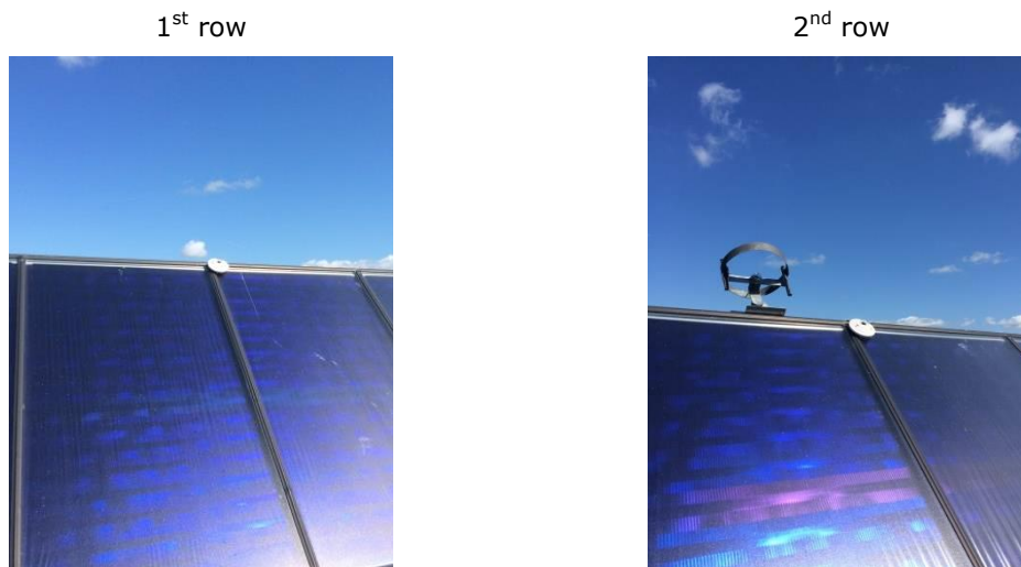
Figure 10. Placement of the pyranometers on the 1 st row and the 2 nd row.
