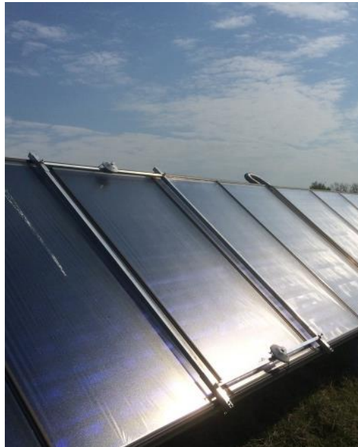
Figure 2. Placement of the pyranometers in fixed positions.
