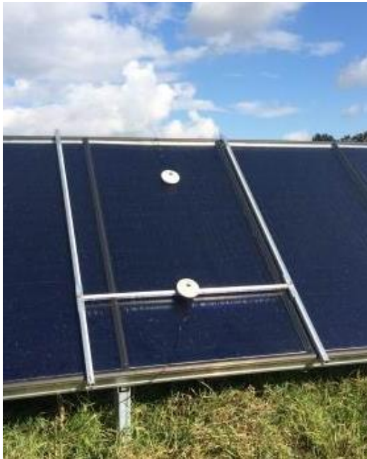
Figure 2. Placement of the pyranometers in fixed positions.
