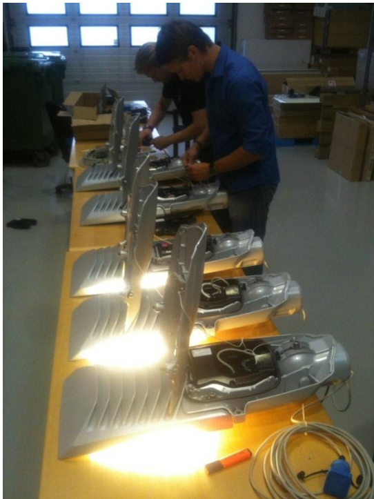
Figur 16: Montering af sensorer i lamper
