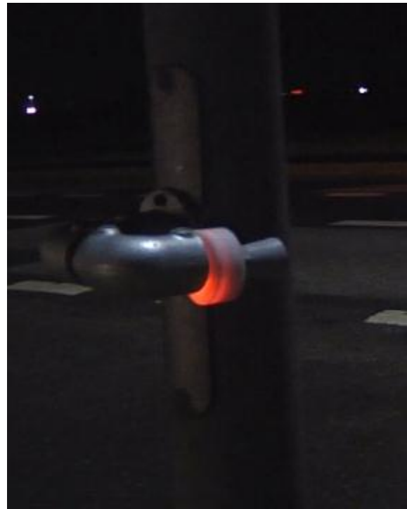
Figur 17: Prototype 2 sensor monteret i mastelugen
