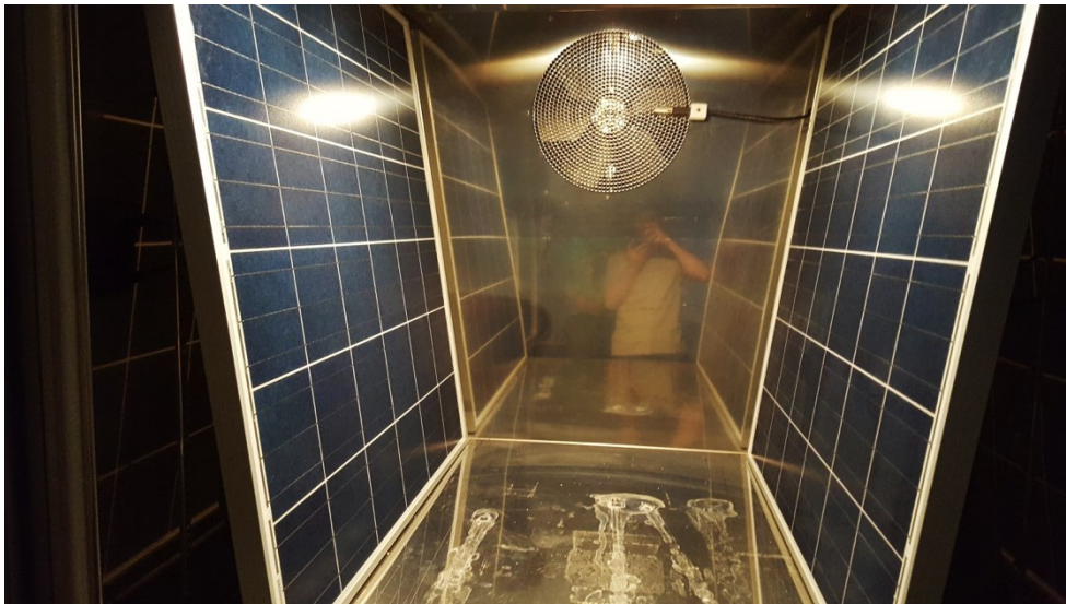
Figure 10: Panels placed in the Angelantoni DY 1200C environmental chamber at AAU, to be undergone humidity-freeze tests.
