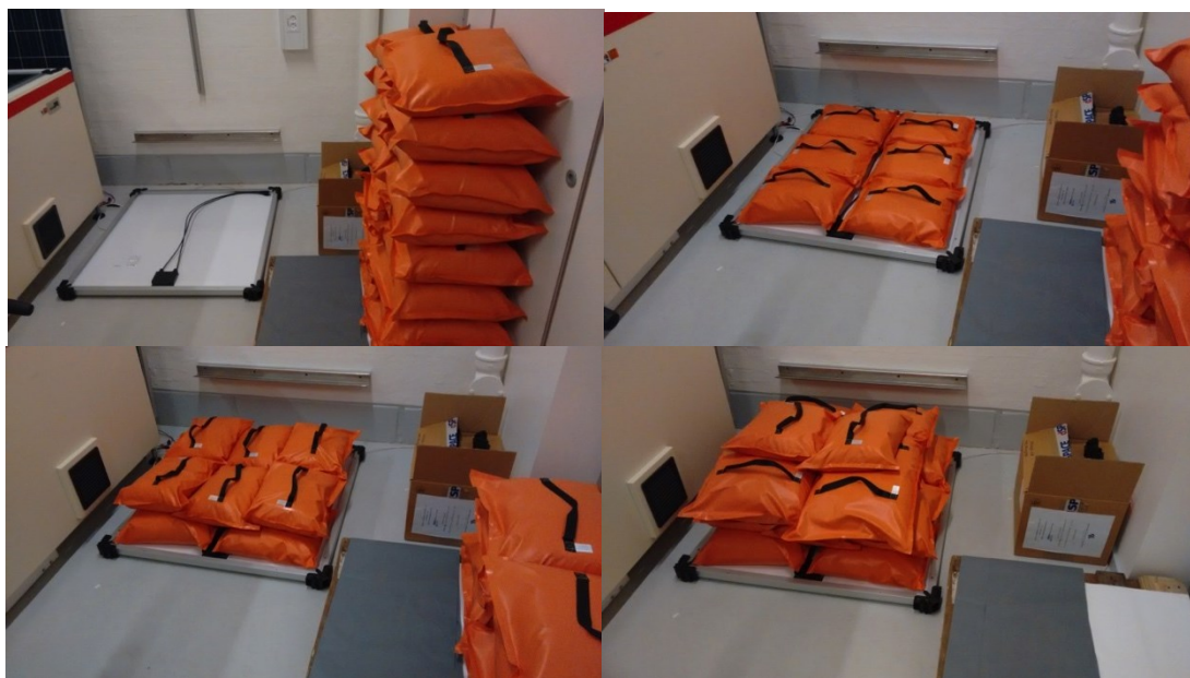
Figure 8: Mechanical loading of the panels to inflict microcracks and cell fractures.
