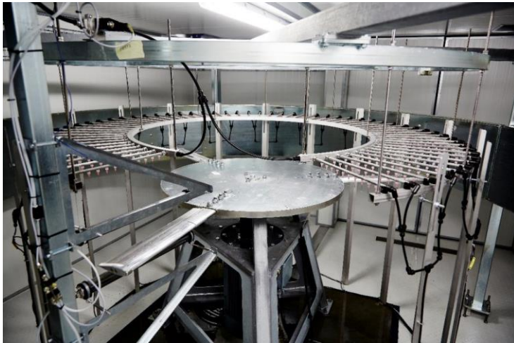
Figure 1: R&D RET unit placed at R&D's head office in Hinnerup, Denmark. Test unit is placed in a double container safely closed during test. The second container is housing the operator control unit, electric installations and water treatment unit. Close-up photo shows a test specimen in the artificial rain field produced in the test unit.
