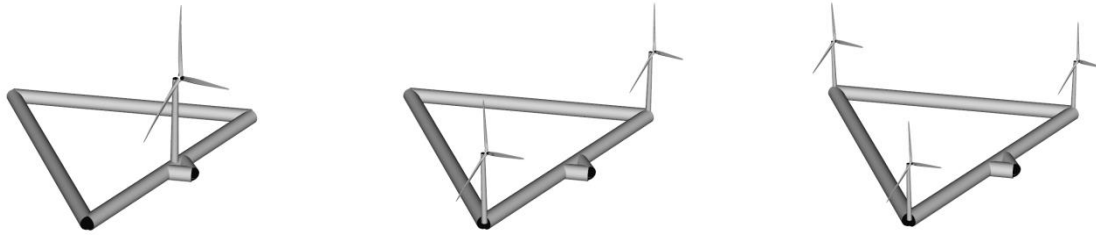
Figure 38 Illustration of three different configurations of installing 10 MW wind power on a floating platform: one 10 MW turbine, two 5 MW turbines or three 3.3 MW turbines.
