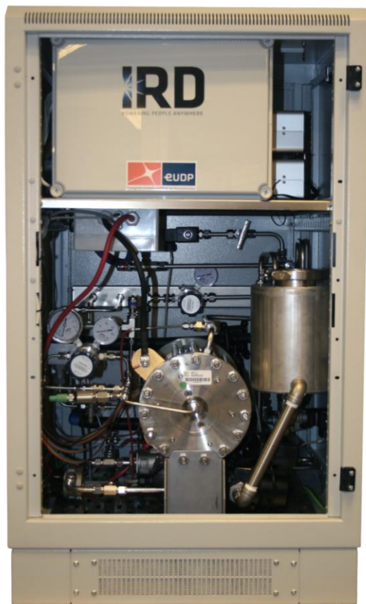
Fig. 19 Picture of the developed \mu PEM electrolyser. The circular PEMEC stack is shown just below the centre of the system.
