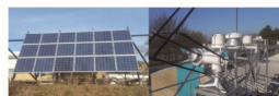
Figure 21: DTU Fotonic, Outdoor PV performance test bed (left) and weather station (right)
