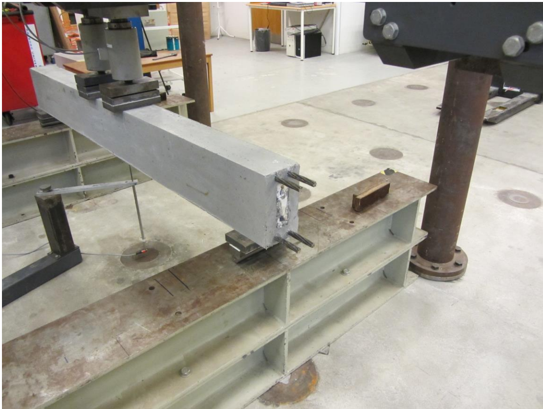
Figure 5 Testing of pre-stressed beam with hollow core.
