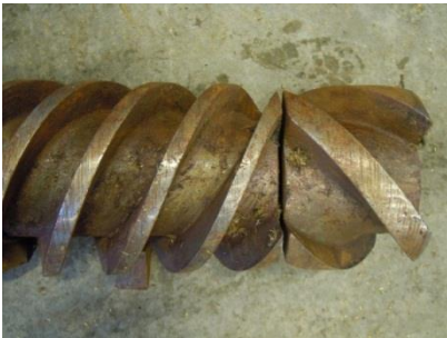
Figure 6. Compression screw element followed by a reverse element (picture of elements for the full-scale extruder)
