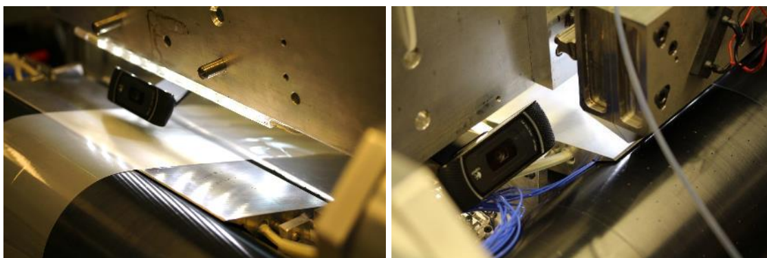
Figure 4: The latest addition to the oven is the small coating plate between the coating drum (black) and glass oven, where immediate drying was possible. Clear wires connects heating elements and blue wires are for temperature sensors. The surface is slightly curved to ensure full contact of the film and it is possible to move the coating head to coat on the first 5 mm of the coating plate. This eliminates any static electricity effects in the gap between the coating drum and the oven.
