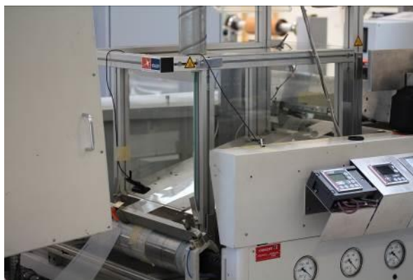
Figure 3: Left: A sketch of the initial oven design, where the foil passes over an aluminium plate, which is heated from the backside using IR lamps. The oven cavity allows for efficient removal of fumes from primarily volatile organic solvents. Right: The oven shown inline after the slot-die coating station.
