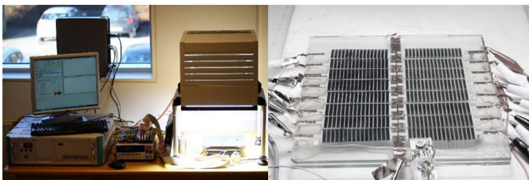
Figure 1: Left: Solar simulator with Keithley IV tracer setup at Mekoprint. Right: A setup of 16 glass-encapsulated modules for extended lifetime testing.
