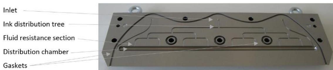
Figure 20: Internal details of prototype coating head.
