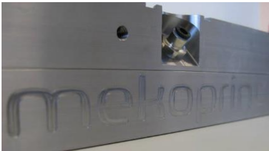
Figure 18: Top picture of the in-house developed and produced prototype coating head. The inlet of ink is seen in the middle.
