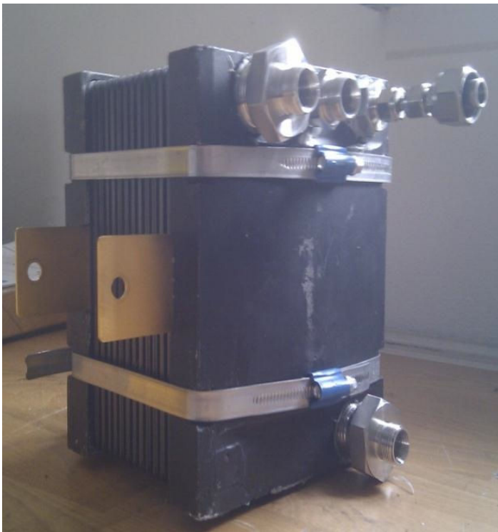
Figure 44. Stack with fiber reinforced high strength concrete composite end plates
