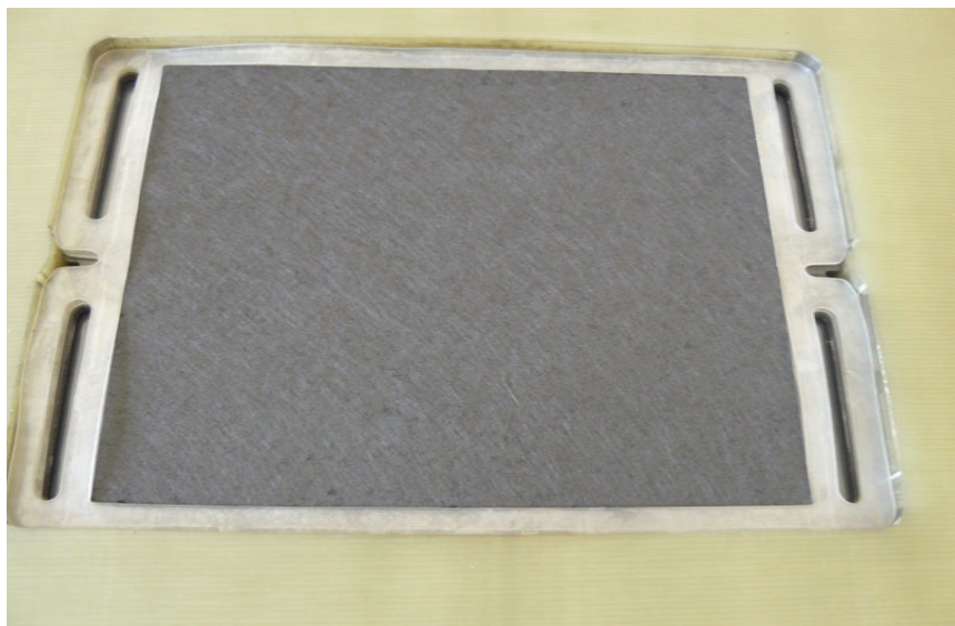
Figure 41. Thermoplastic flat sealing of MEA/flow plate
