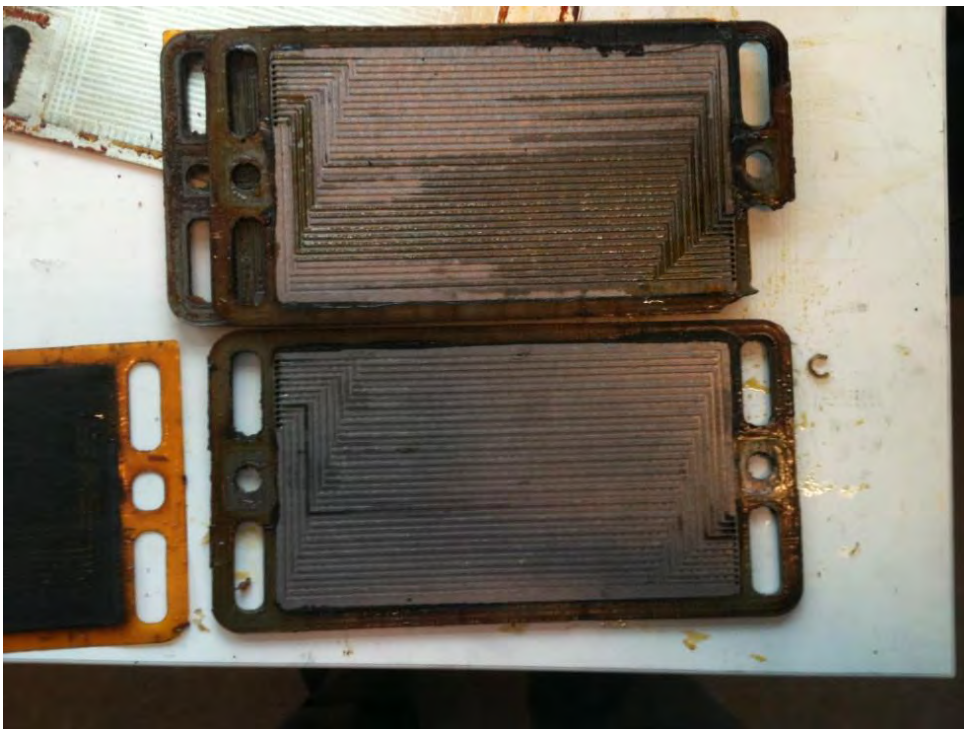
Figure 3: Acryl gaskets after 1500hr of operation.
