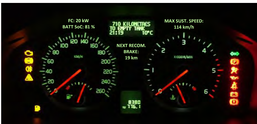
Picture 3 – Possible layout of an updated dashboard for an electric vehicle with a HI-EPS
