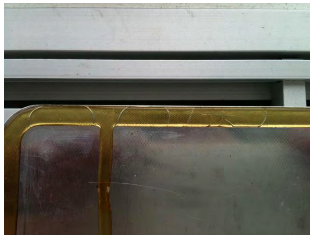
Figure 2: Acryl gasket after 2 hours in a oven at 240°C.
