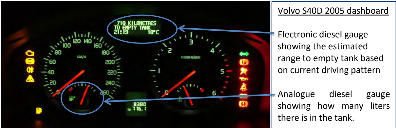
Picture 2 – Dashboard of a never car with both an analogue and a digital diesel gauge
