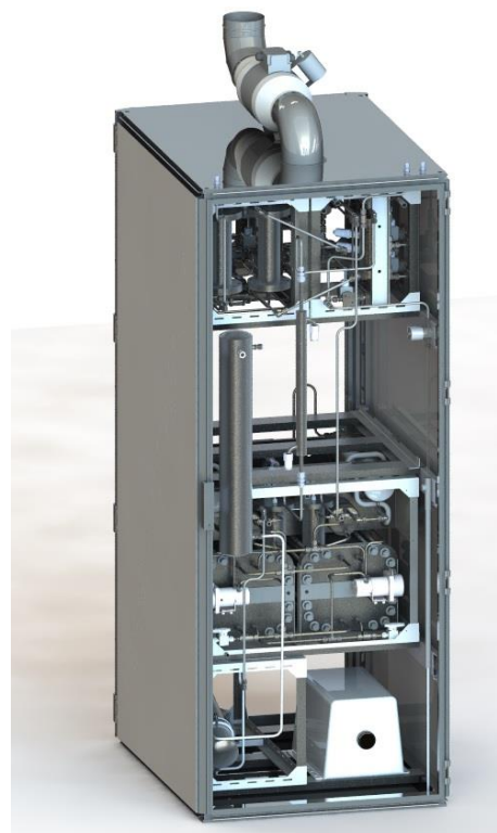
Figure 10: Prototype of entire electrolyser system
