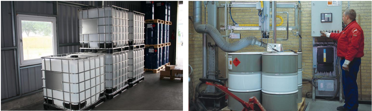
Figure 9: 1000 L tanks & 250 L drums (left), mixing and tapping equipment (right)
