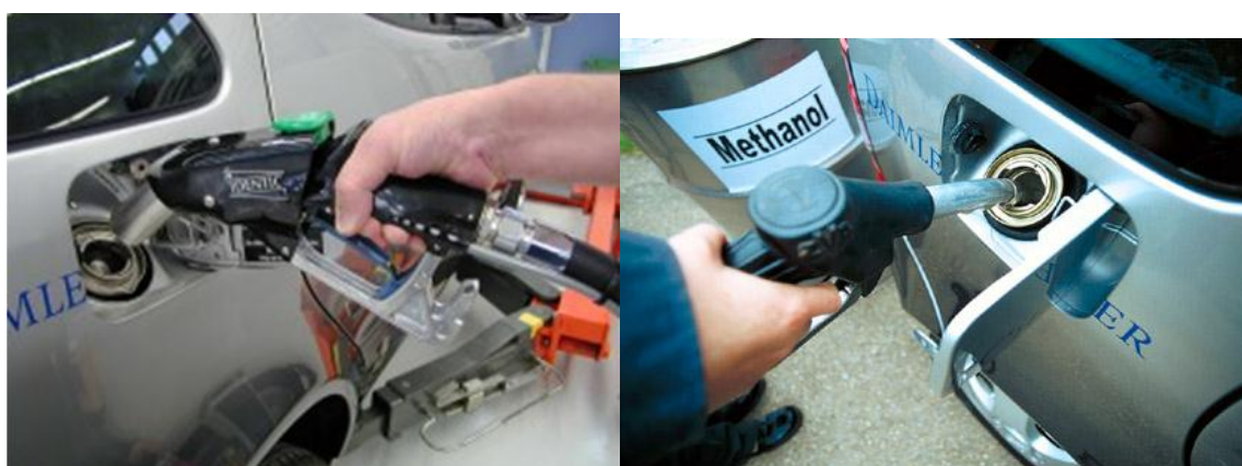
Figure 40: The old and the new dispensing system for the NECAR 5
