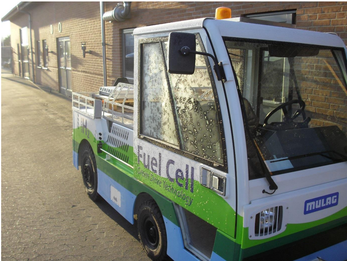
Climate tests of MULAG 3FC in Winter @ -13°C.
