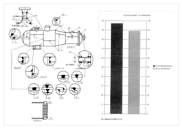
The figure below shows the final design for a 35MPa storage vessel.
