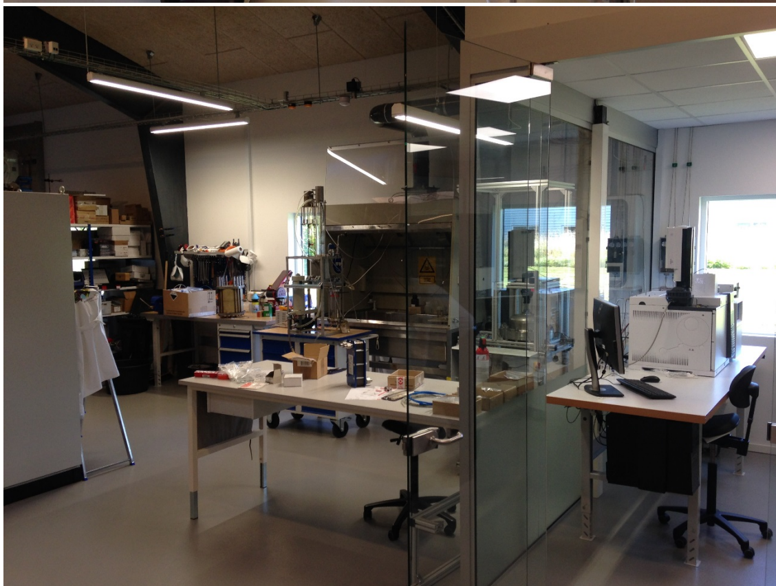
Figure 2: The gas laboratory in Horsens. The fume cabinet is used for the experiments with the gas cleaning systems. The gas chromatograph can be viewed in the bottom right corner, close to the working area, but safely behind glass as to ensure no accidents are to harm it.
