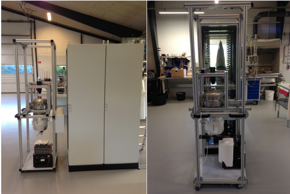
Figure 10: The reactor with the enclosing made to resemble that of the final design, i.e. the cabinets next to the enclosing. In the final design, several reactors will be in the same cabinet.
