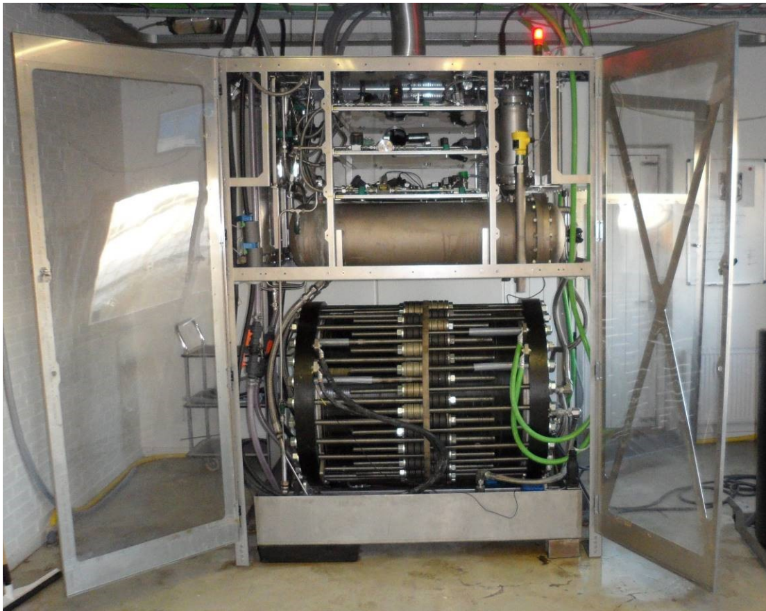
Figure 11. Prototype of a 60 Nm 3 /h alkaline electrolyser unit developed within the project "HyProvide Large-Scale Alkaline Electrolyser (MW)" during the years 2011 to 2015.
