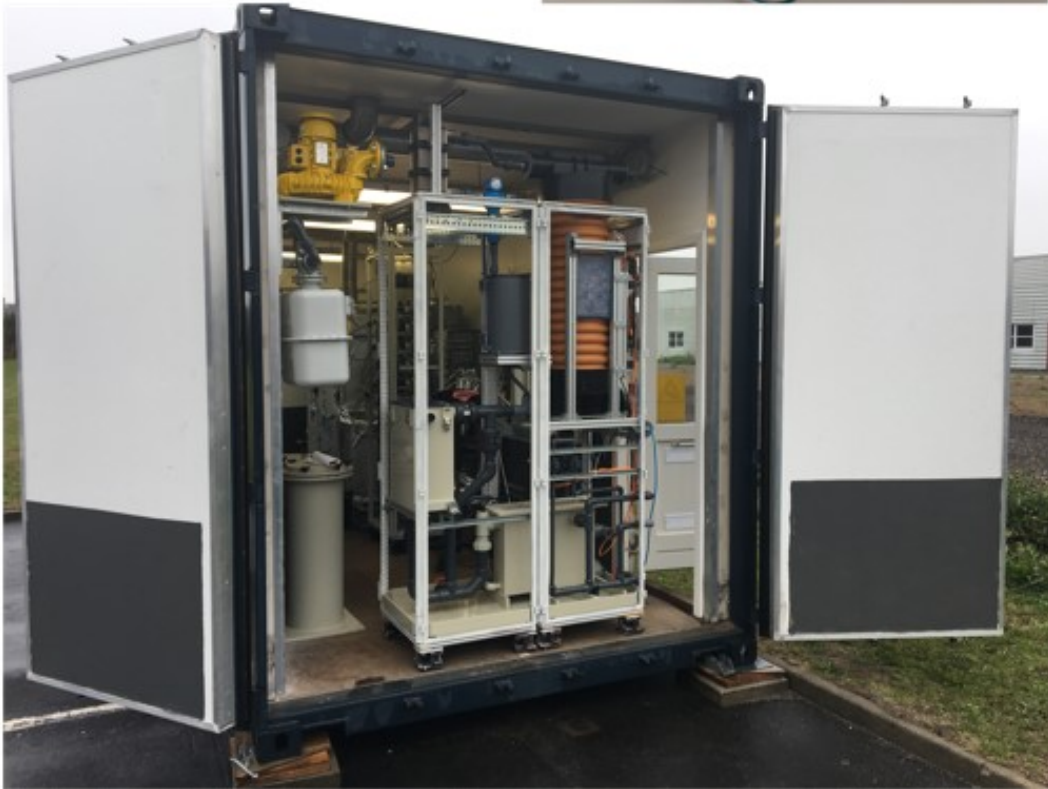
Figure 7: The biogas desulfurization units constructed and tested during the MeGa-StoRE project by PhD Student Sebastian Nis Bay Villadsen. a) The first unit constructed within 1 month of initializing the PhD project. b) The first unit to be tested on authentic biogas at a biogas plant. c) The unit is currently being tested at the Midtfyn biogas plant.
