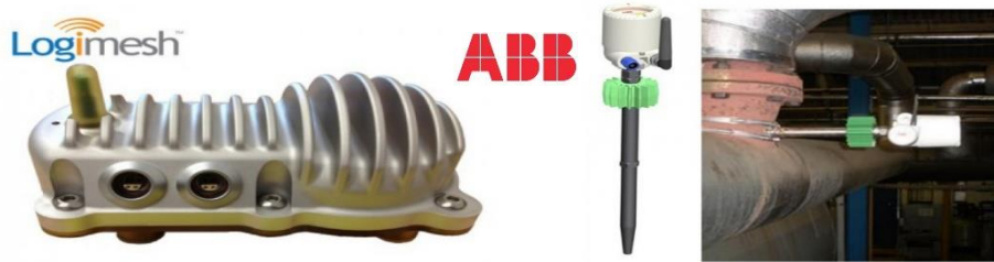
Figure 6 Wireless sensors powered by TEGs. Logimesh’s vibration sensor and ABB’s temperature sensor. Both products are commercially available today.
