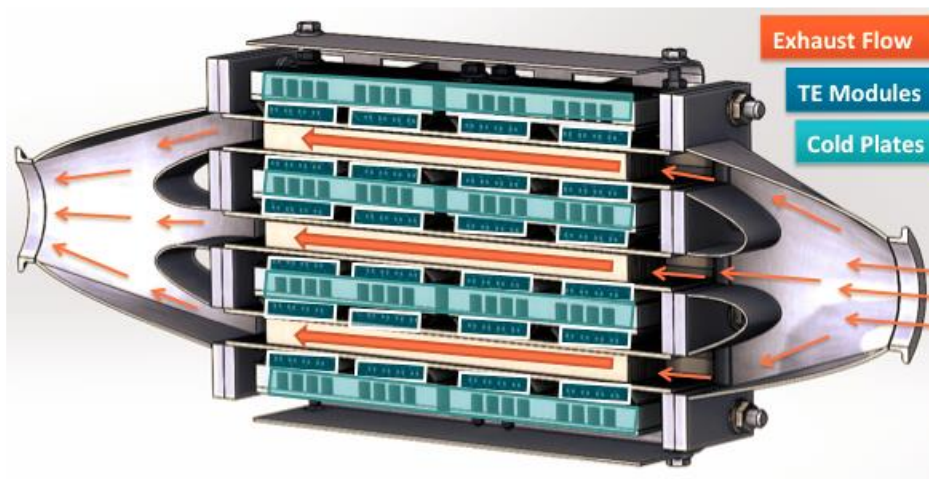
Figure 11 Exhaust gas heat exchanger. The exhaust gas passes through channels in close thermal contact with the TEG's hot side. Cooling water passes through channels in close thermal contact with the TEG's cold side. From [8].
