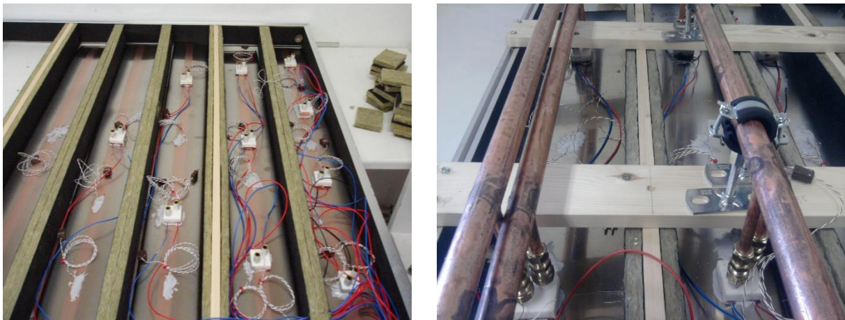
Figure 13 Details of the H1 hybrid solar collector. Picture to the left shows TEGs mounted directly on the back-side of the solar absorber using Danfoss ShowerPower modules. Picture to the right shows the interconnection of the cooling circuit to the ShowerPower modules.
