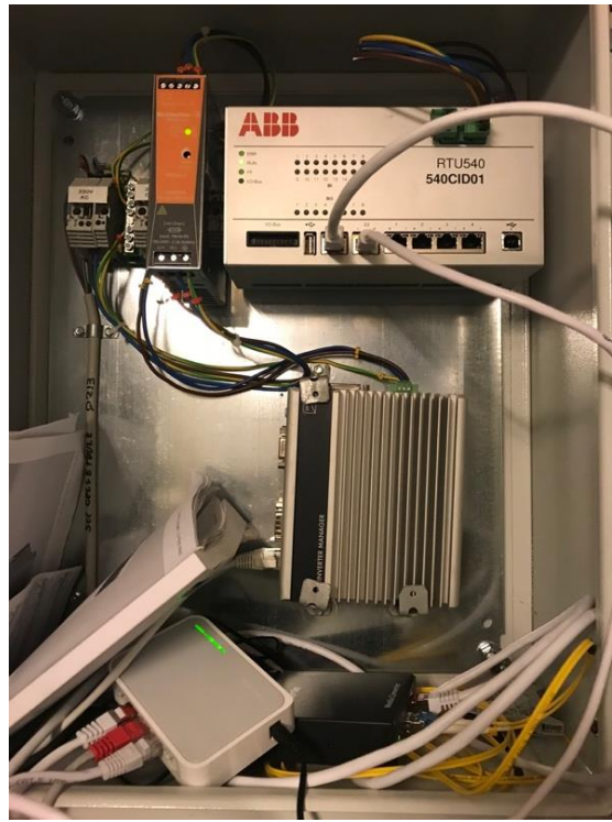
Photo 1. Setup of the RTU and measurement system at campus
